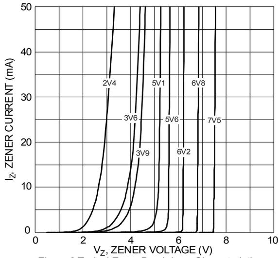
Figure 3 Typical Zener Breakdown Characteristics
