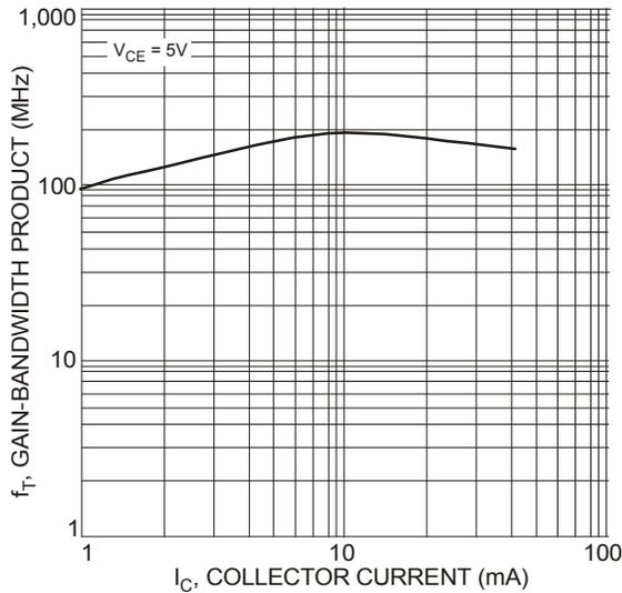
Figure 3 Typical Gain-Bandwidth Product vs. Collector Current
