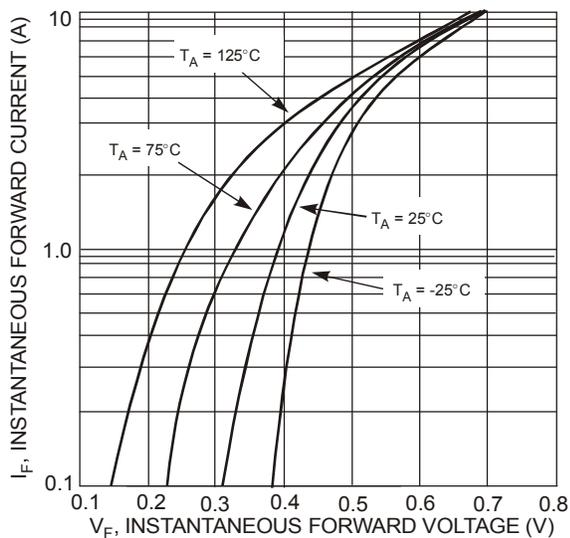
Figure 1 Typical Forward Characteristics - B320B thru B340B
