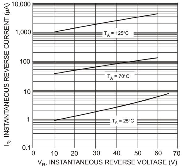
Figure 4 Typical Reverse Characteristics, B350B thru B360B
