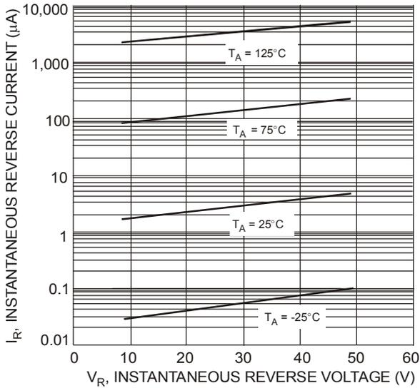
Figure 3 Typical Reverse Characteristics, B320B thru B340B
