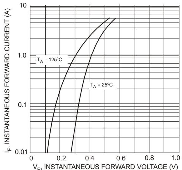
Figure 2 Typical Forward Characteristics - B350B thru B360B
