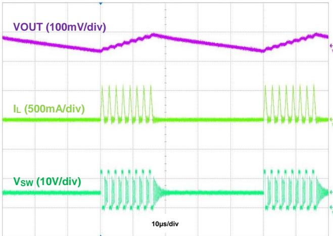
Figure 14. Output Voltage Ripple,  $I_{OUT} = 50\text{mA}$
