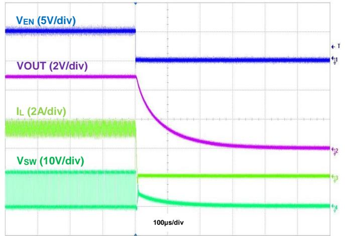
Figure 20. Shutdown Using EN,  $I_{OUT} = 3.5\text{A}$
