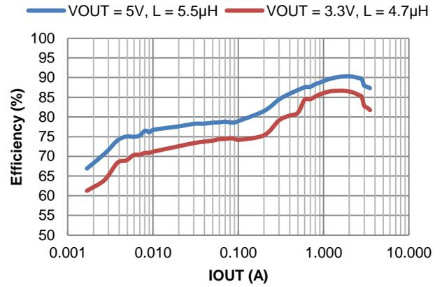
Figure 5. Efficiency vs. Output Current,  $V_{IN} = 24\text{V}$
