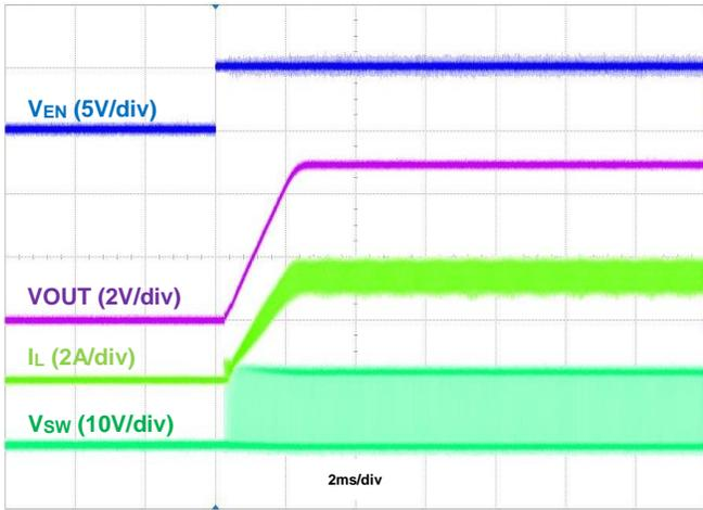
Figure 19. Startup Using EN,  $I_{OUT} = 3.5\text{A}$
