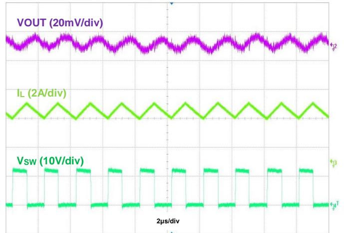
Figure 15. Output Voltage Ripple,  $I_{OUT} = 3.5\text{A}$
