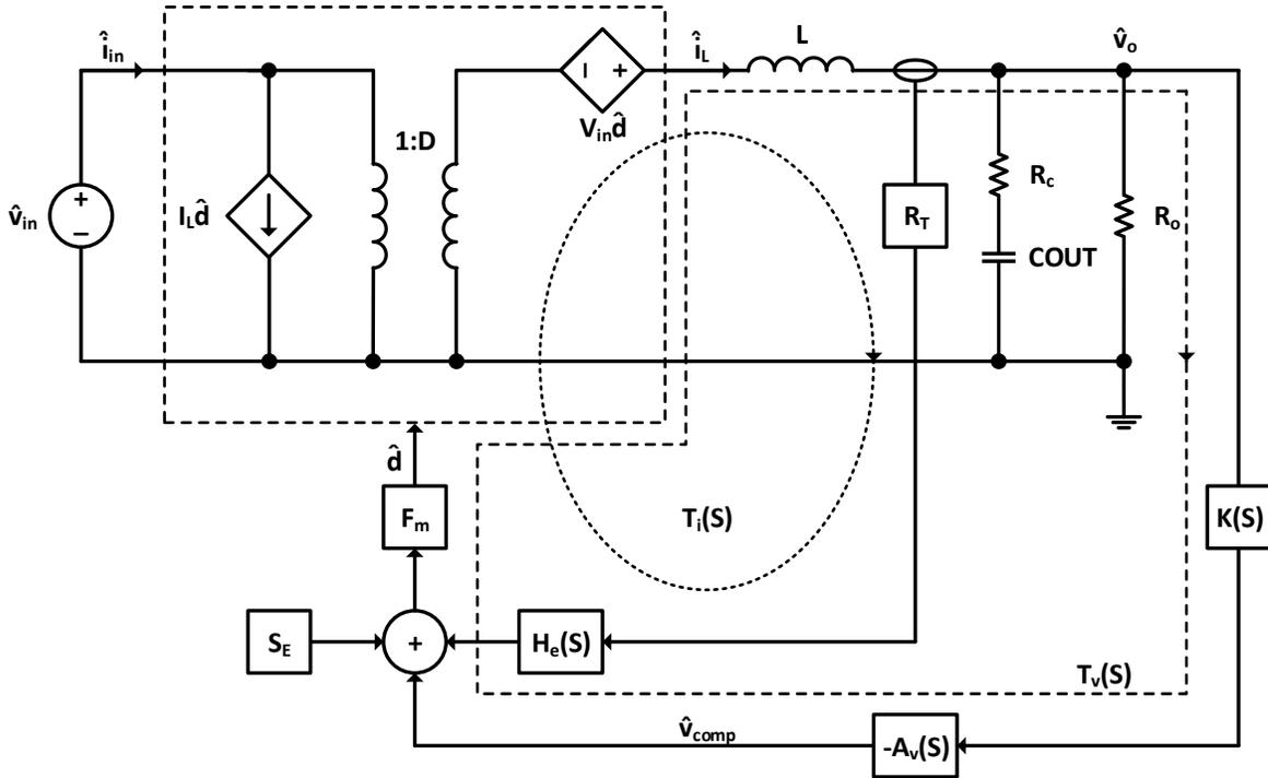
Figure 26. Small Signal Model of Buck Regulator
