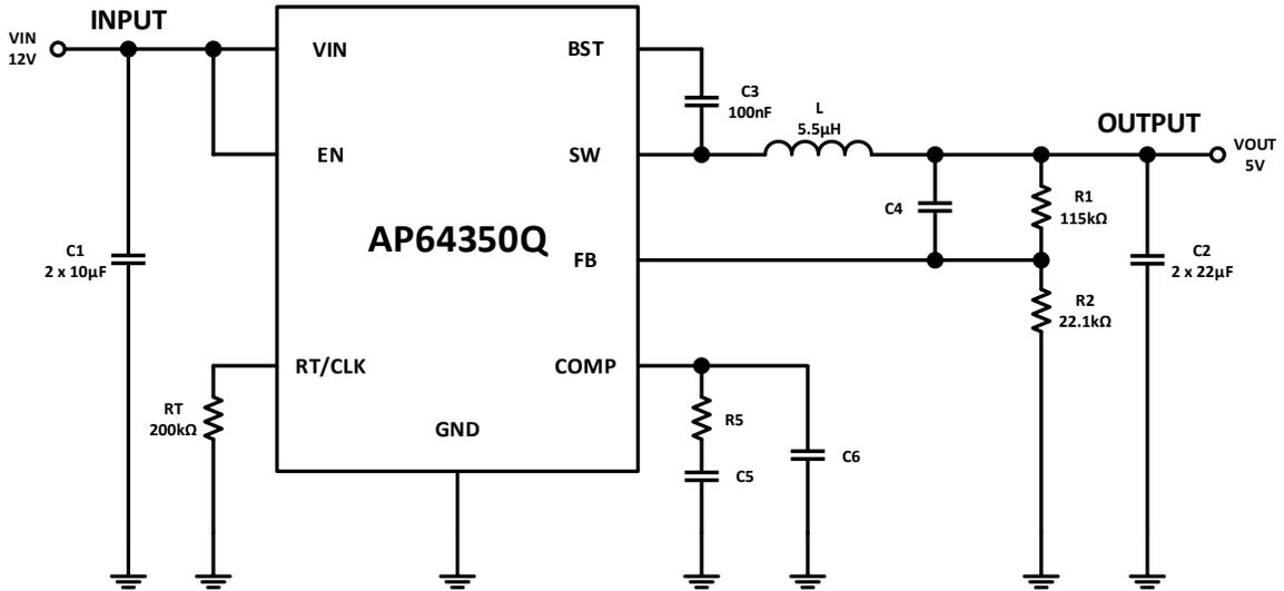
**Figure 28. Example Circuit for Loop Compensation Calculations**
