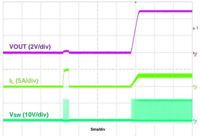
Figure 22. Output Short Recovery,  $I_{OUT} = 3.5\text{A}$
