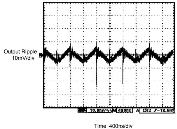
**Output Ripple @  $V_{IN} = 2.7V$ ,  $I_{OUT} = 100mA$**
