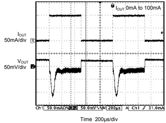
**Output Ripple @  $V_{IN} = 2.7V$ ,  $I_{OUT} = 0mA$**
