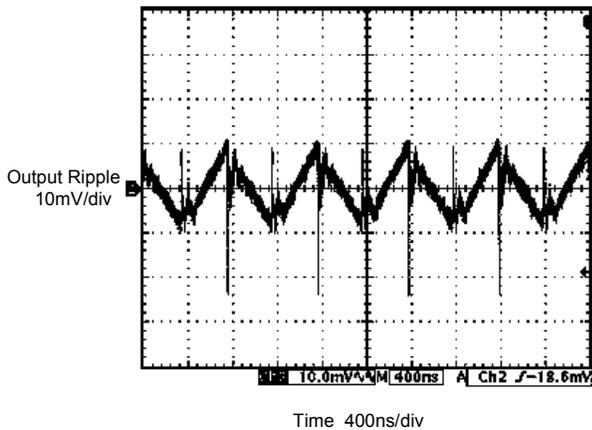
**Performance Characteristics** (cont.) (Unless otherwise noted,  $V_{IN} = 3.0V$ ,  $C_{IN} = C_{OUT} = 10\mu F$ ,  $C_{FLY} = 1\mu F$  Ceramic Cap,  $T_A = +25^\circ C$ )
