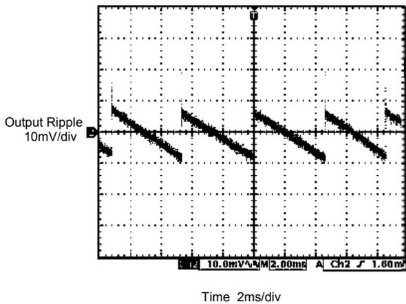
**Output Ripple @  $V_{IN} = 2.7V$ ,  $I_{OUT} = 50mA$**
