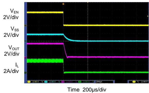
**Short Circuit Protection ( $I_{OUT}=3\text{A}$ )**
