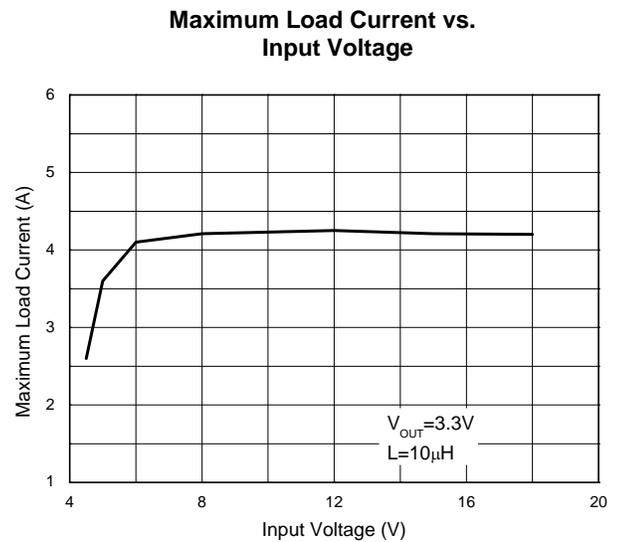
**Performance Characteristics** (Cont.  $T_A=+25^{\circ}\text{C}$ ,  $V_{IN}=12\text{V}$ ,  $V_{OUT}=3.3\text{V}$ , unless otherwise noted.)
