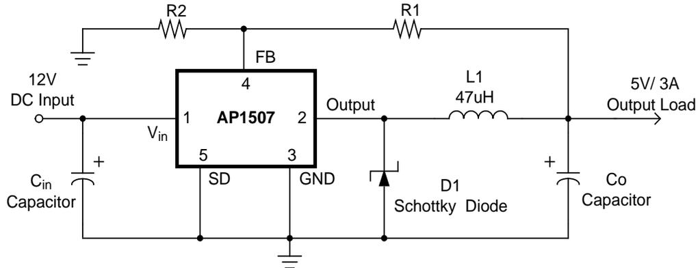
$$V_{OUT} = V_{FB} \times \left(1 + \frac{R1}{R2}\right)$$
