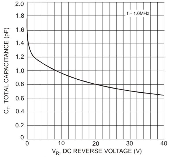
Fig. 4 Typical Total Capacitance vs. Reverse Voltage
