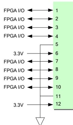
Figure 12 - Pmod Connections
