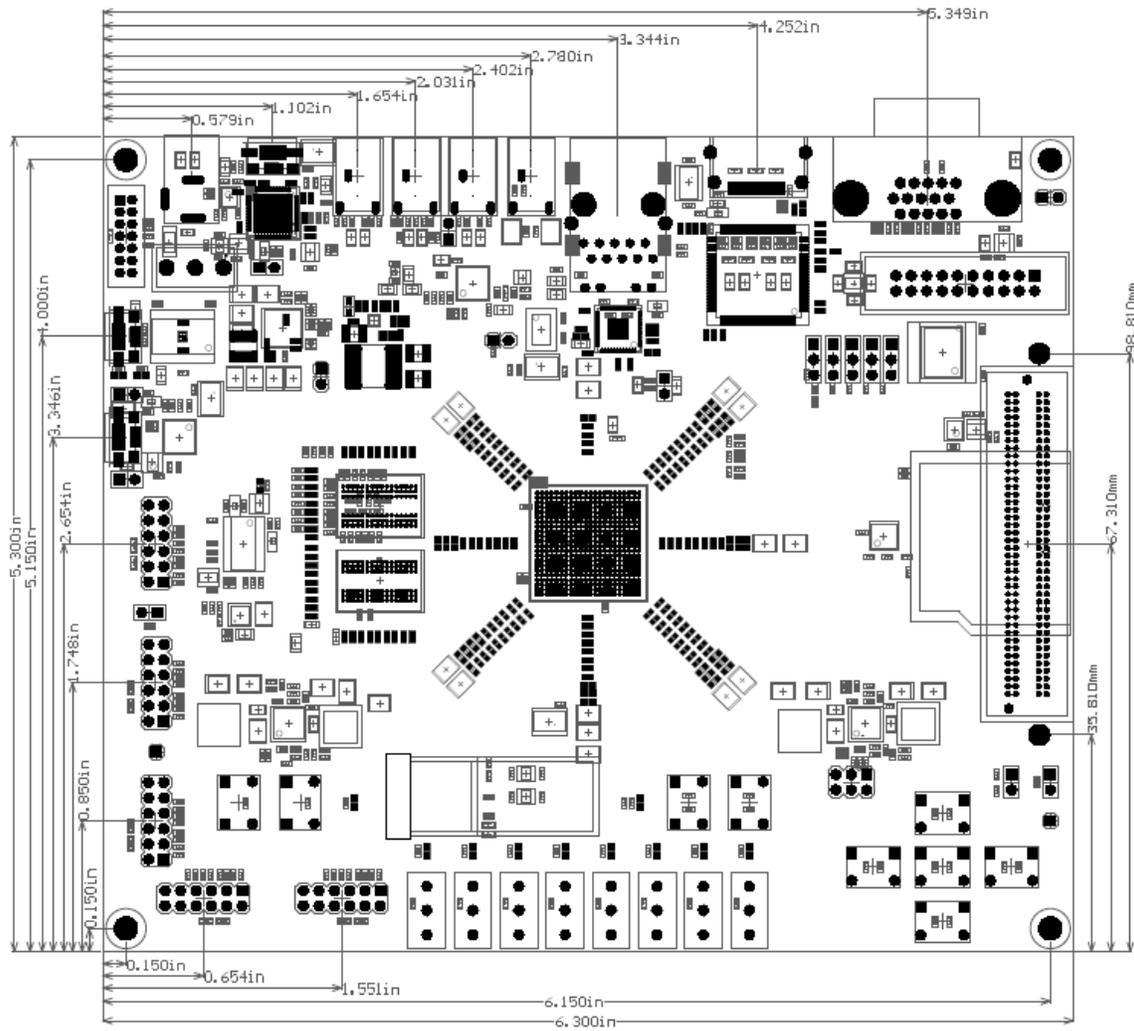
Figure 21 - ZedBoard Mechanical
