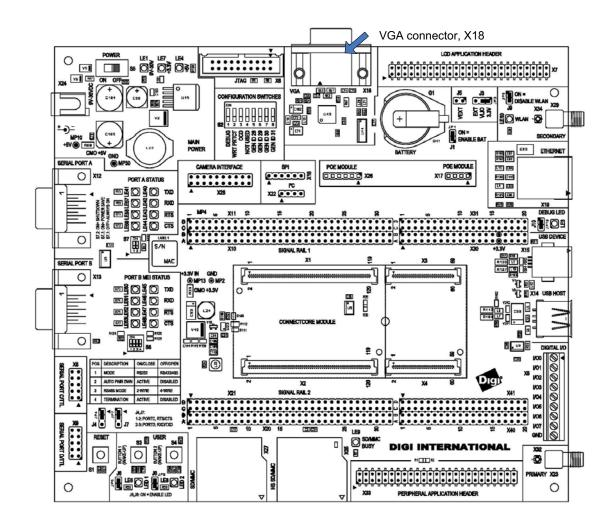
VGA connector, The VGA connector is a 15-pin female connector, labeled X18. X18
