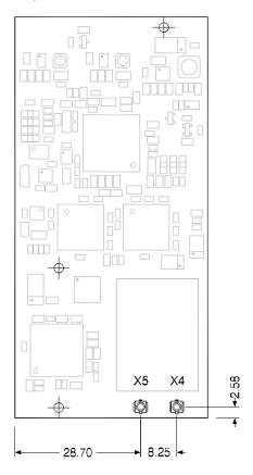
Note When disconnecting U.FL connectors, the use of U.FL plug extraction tool (Hirose P/N U.FL-LP-N-2 or U.FL-LP(V)-N-2) is strongly recommended to avoid damage to the U.FL connectors on the ConnectCore Wi-9M 2443 module.
