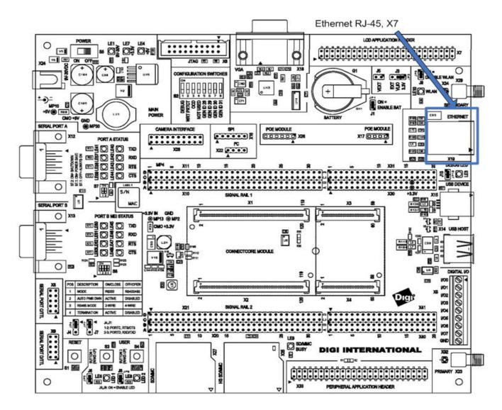
The module provides the 10/100 Ethernet MAC and PHY chip. The development board provides the 1:1 transformer and Ethernet connector.
