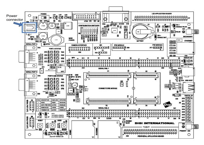
The power connector is a barrel connector with a 9-30VDC operating range. The power jack is labeled X24 on the development board. The figure below represents the power jack polarity.
