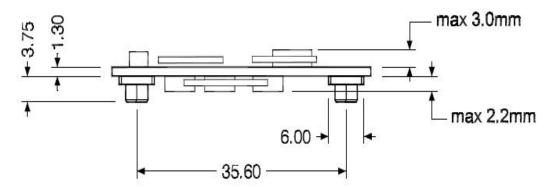
The module measures  $60 \times 44$ mm. Two holes are provided for M2 screws to enable secure mounting of the module on the base board.
