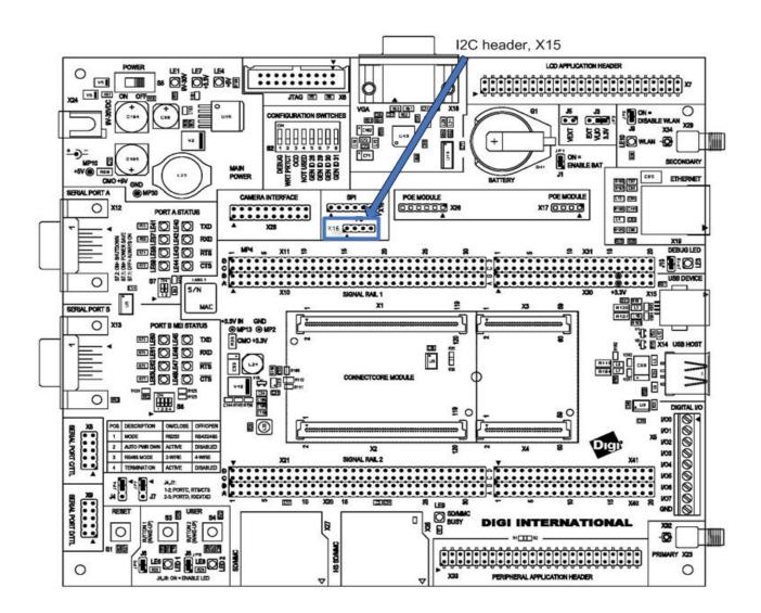
I2C connector, X15 The table below provides the pinout of the I2C header.
