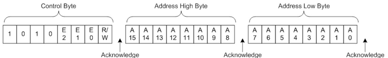
The device will acknowledge each byte of data that is received by pulling the SDA line low during the 9th clock pulse. If the device does not provide an acknowledge, it has not received the data; consequently the entire sequence, starting with the control byte, must be resent.
