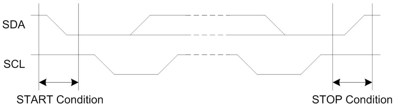
Every byte put on the SDA line must be 8 bits long. The number of bytes that can be transmitted per transfer is unrestricted. Each byte must be followed by an acknowledge bit; therefore, the number of clock cycles to transfer one byte is nine. Data is transferred with the most significant bit (MSB) first.
