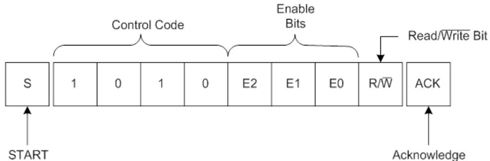
Upon receiving a "1010", the chip enable bits, and the  $\overline{R/W}$  bit, the device performs an acknowledge by pulling the SDA line low during the 9th clock pulse. As stated above, the device will now be set for either a read or a write operation by the  $\overline{R/W}$  bit.
