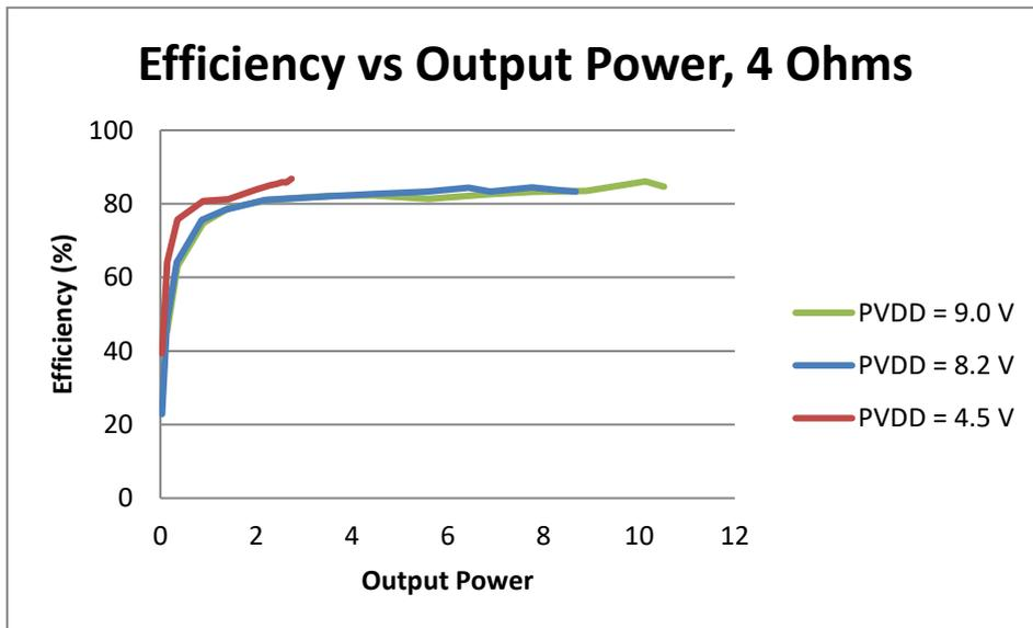
Figure 14: Efficiency versus output power (4 Ω + 33 μH)
