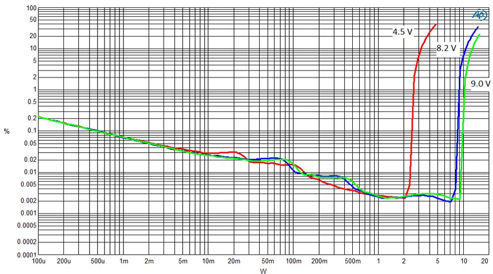
Figure 4: THD versus output power (4 Ω + 33 μH)
