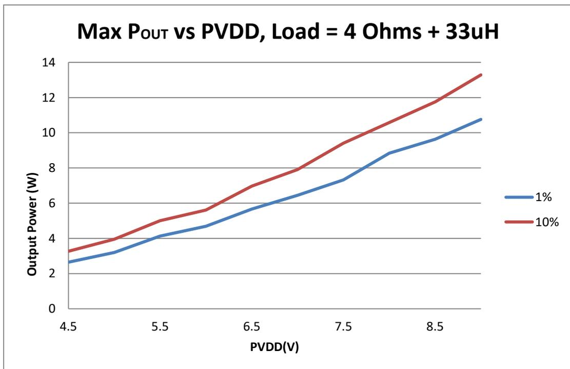
Figure 12: Maximum output power (P<sub>out</sub>) versus supply voltage (4 Ω + 33 μH)
