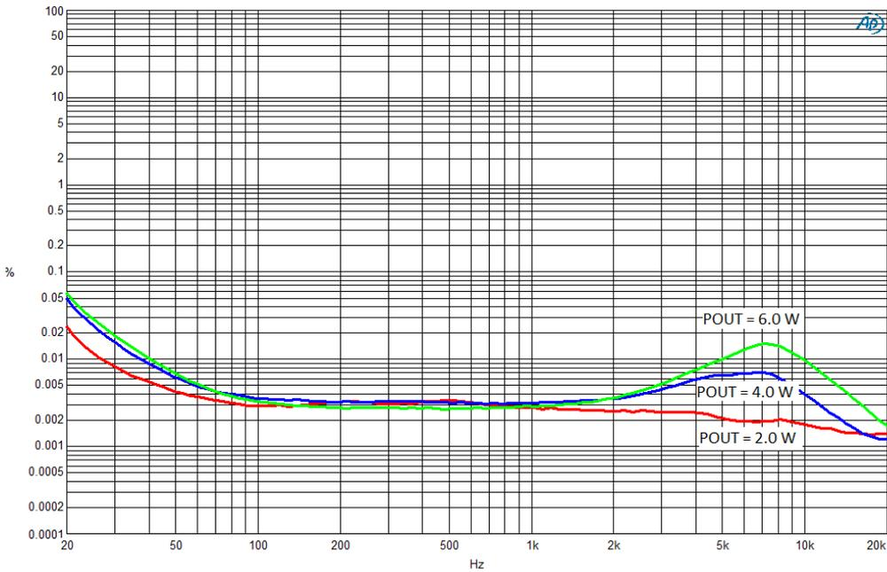
Figure 10: THD versus frequency (4 Ω + 33 μH) 9.0 V
