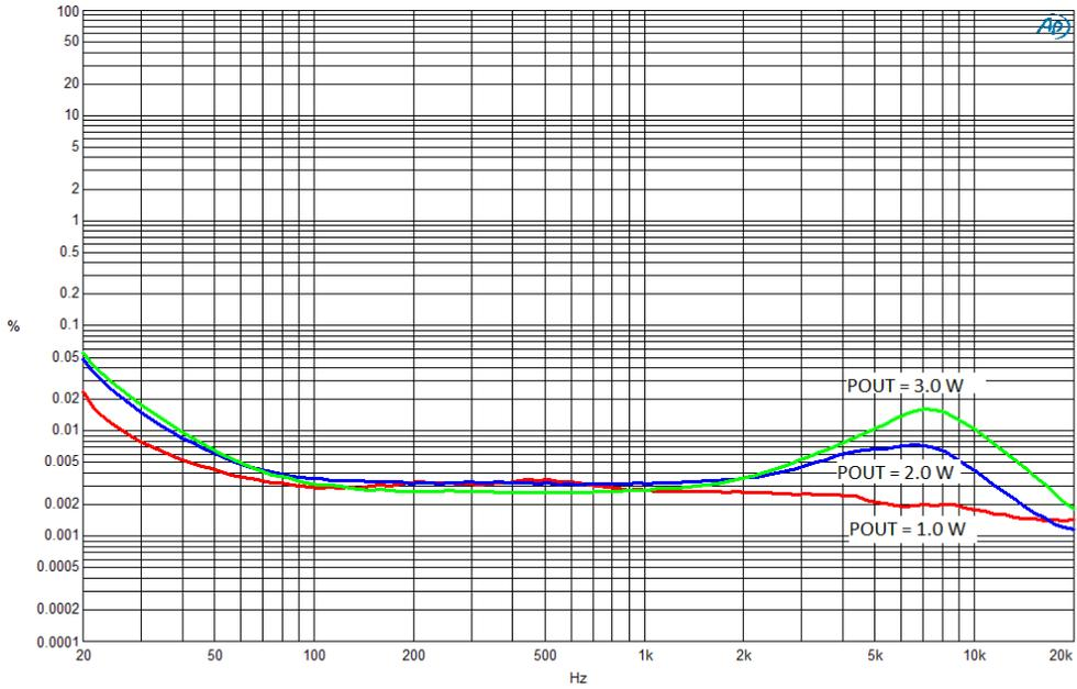
Figure 9: THD versus frequency (8 Ω + 33 μH) 9.0 V
