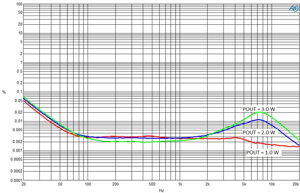
Figure 7: THD versus frequency (8 Ω + 33 μH) 8.2 V
