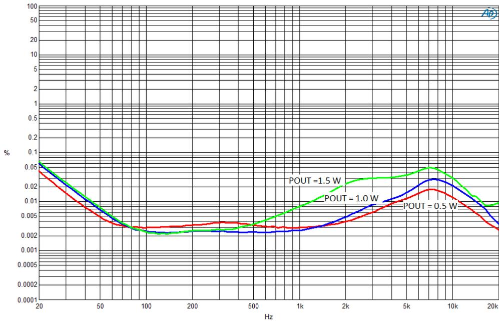
Figure 5: THD versus frequency (8 Ω + 33 μH) 4.5 V
