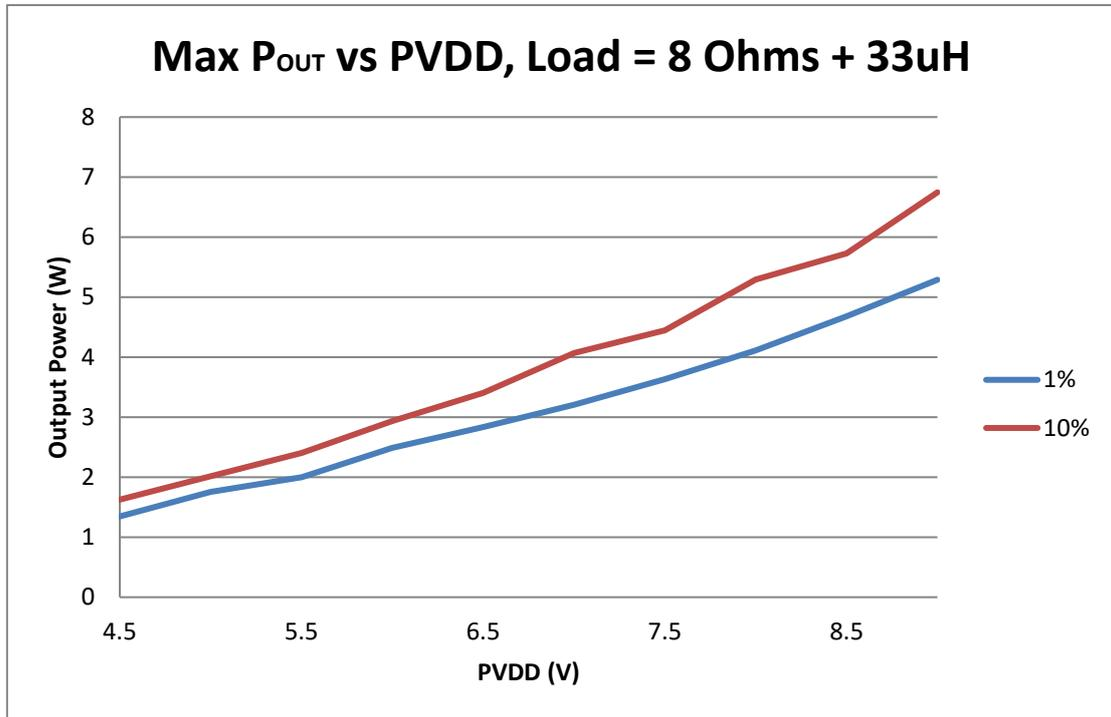
Figure 11: Maximum output power (P<sub>out</sub>) versus supply voltage (8 Ω + 33 μH)
