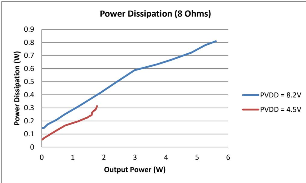
Figure 17: Power dissipation versus output power (8 Ω + 33 μH)
