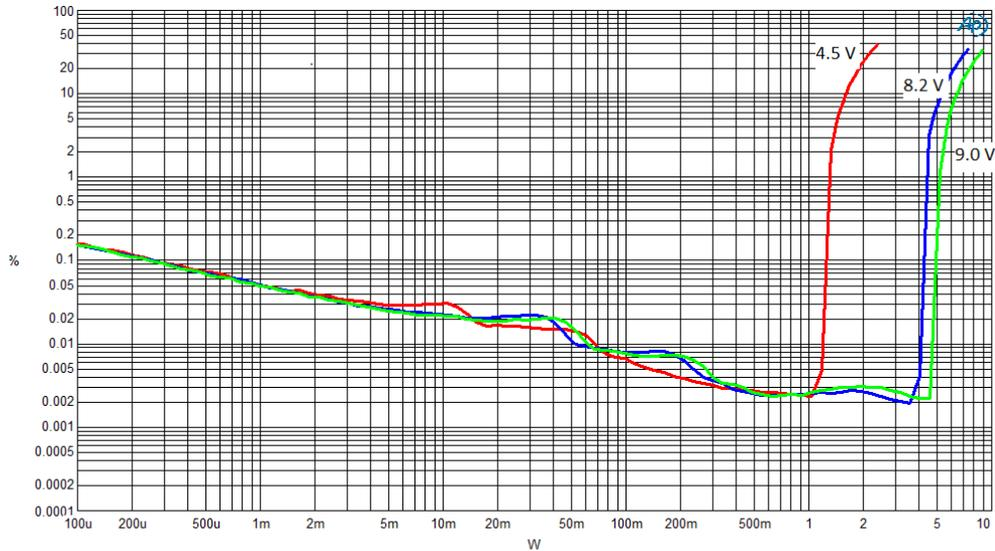
Figure 3: THD versus output power (8 Ω + 33 μH)
