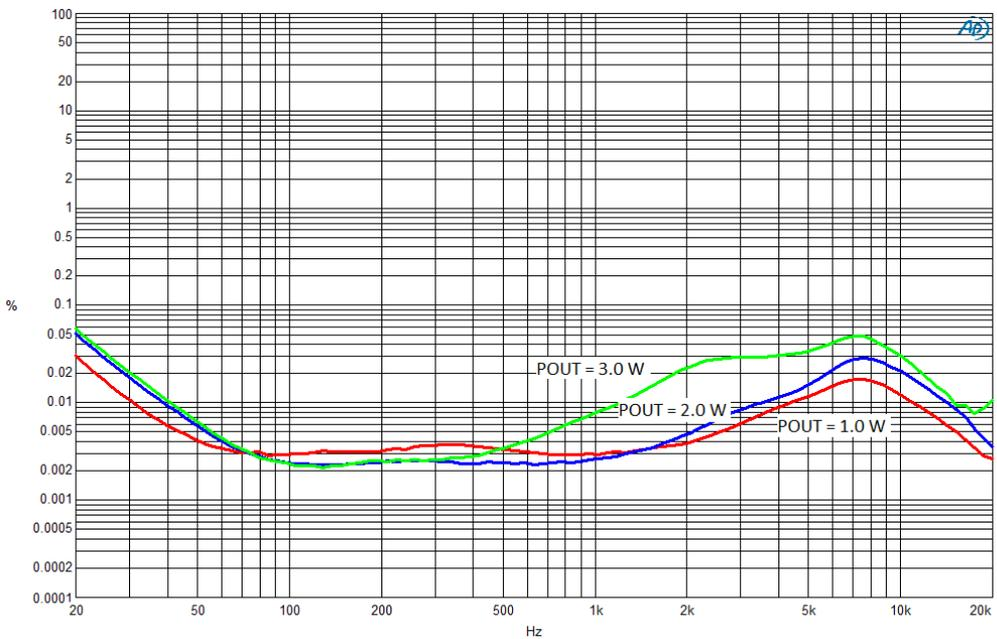
Figure 6: THD versus frequency (4 Ω + 33 μH) 4.5 V
