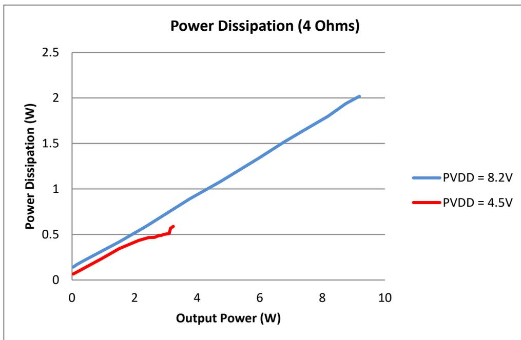
Figure 18: Power dissipation versus output power (4 Ω + 33 μH)
