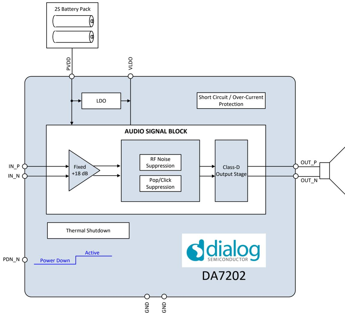
Figure 1: DA7202 block diagram
