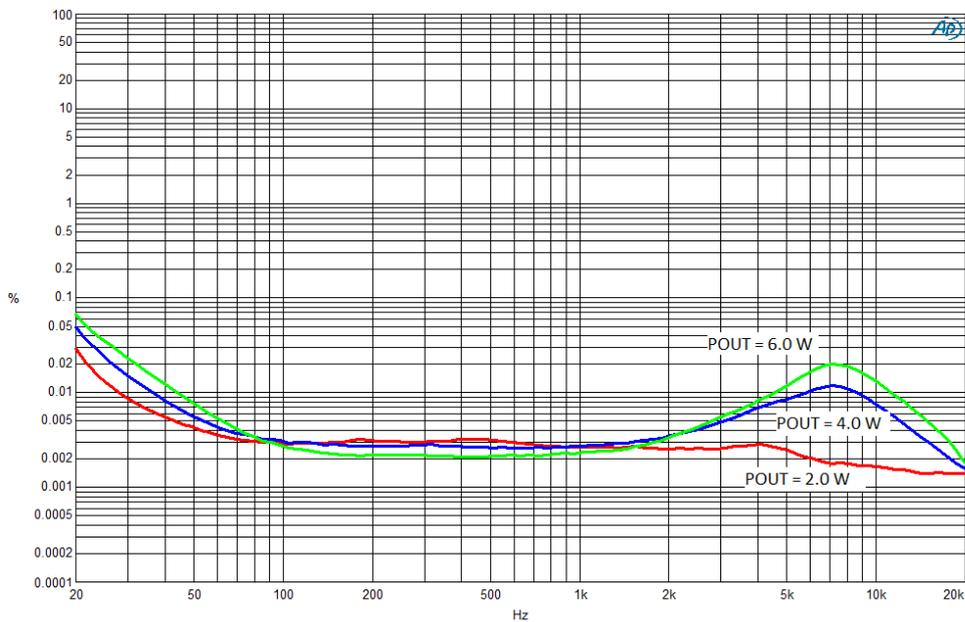
Figure 8: THD versus frequency (4 Ω + 33 μH) 8.2 V
