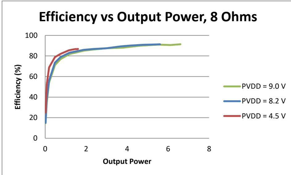
Figure 13: Efficiency versus output power (8 Ω + 33 μH)
