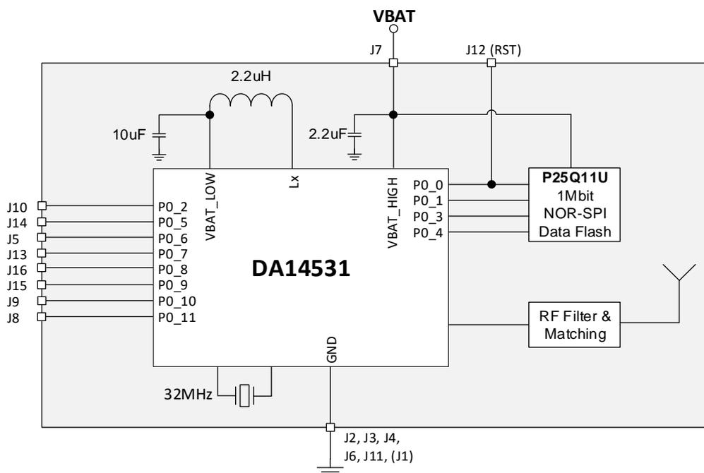
Figure 1: DA14531 SmartBond TINY™ Module Block Diagram
