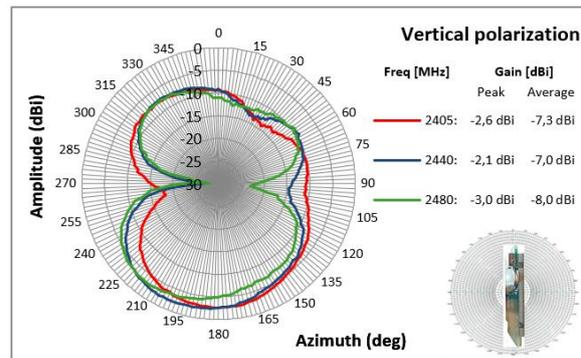
Figure 18: Radiation Pattern for XZ-Plane, Vertical Polarization
