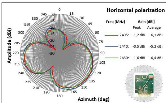
Figure 19: Radiation Pattern for YZ-Plane, Horizontal Polarization
