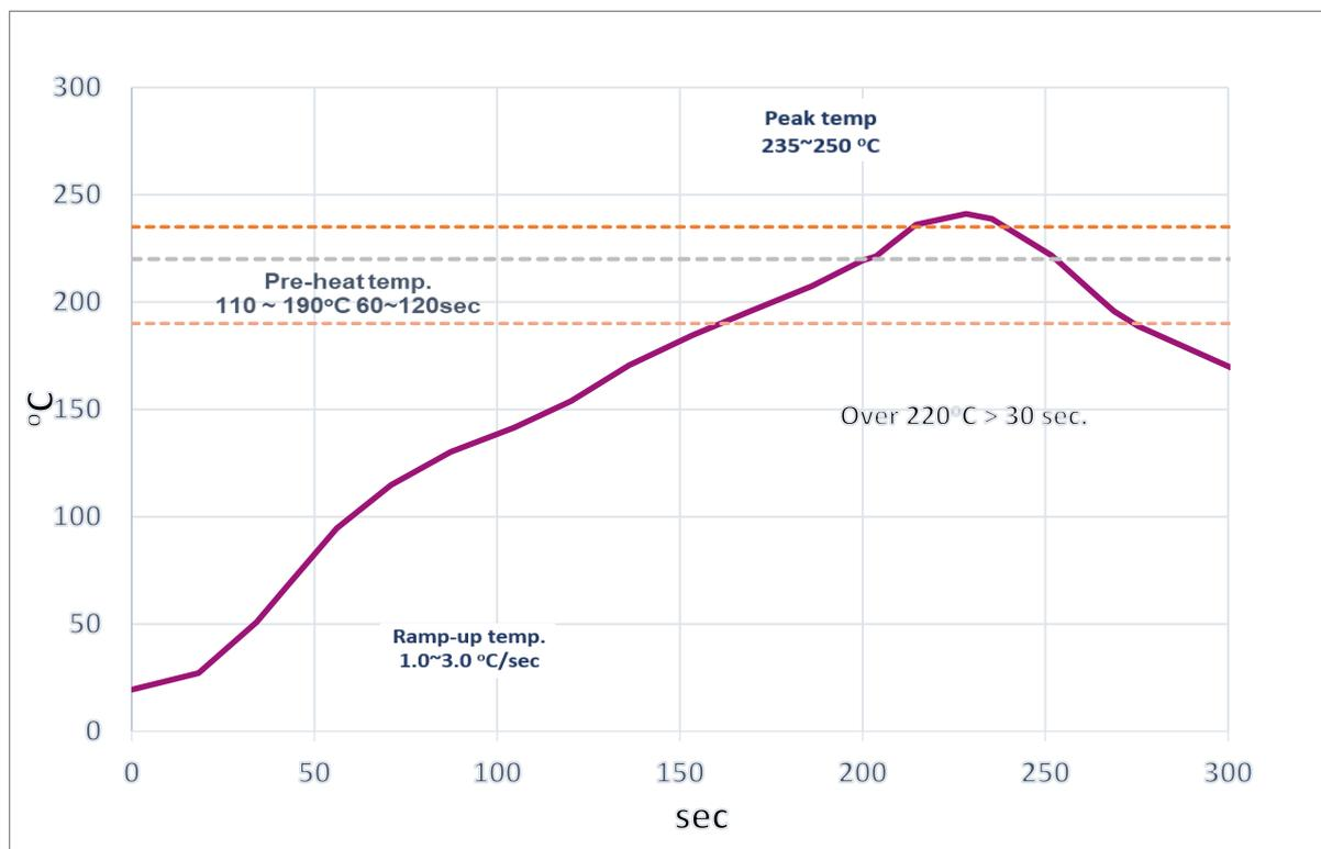
Figure 21: Recommended Reflow Profile for Lead Free Solder
