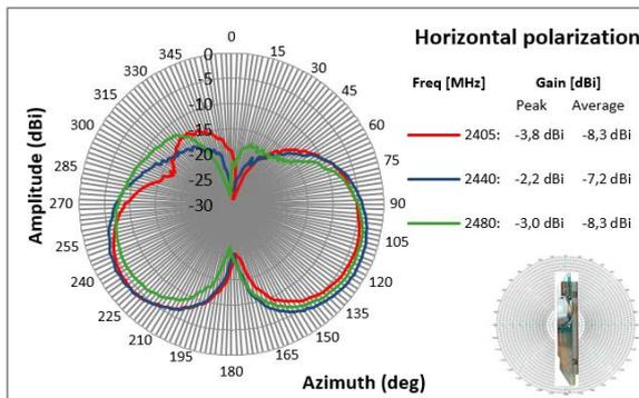
Figure 17: Radiation Pattern for XZ-Plane, Horizontal Polarization
