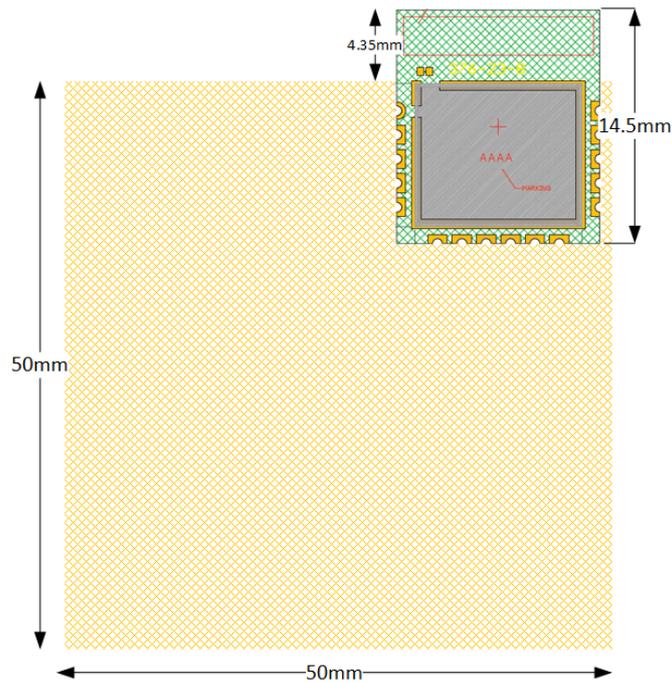
**Figure 10: DA14531 TINY™ Module Evaluation Board**
