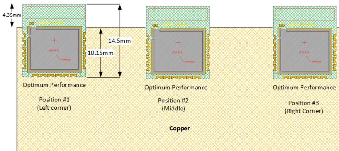
**Figure 8: Installation Locations for Optimum Antenna Performance**
