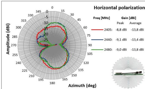
Figure 15: Radiation Pattern for XY-Plane, Horizontal Polarization
