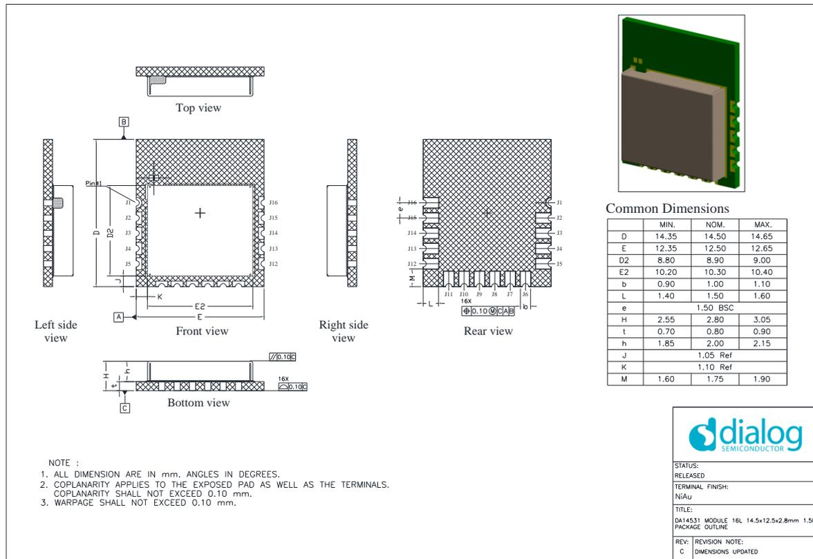
Figure 3: Mechanical Drawing
