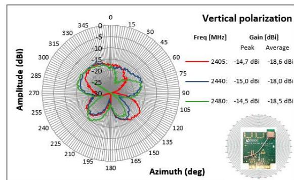
Figure 20: Radiation Pattern for YZ-Plane, Vertical Polarization
