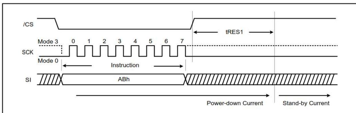
Figure 7-40. Release Power Down Instruction (QPI Mode)
