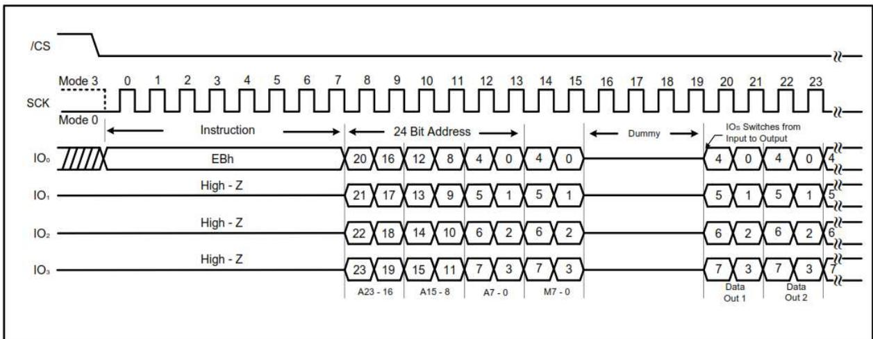
Figure 7-19. Fast Read Quad I/O Instruction (previous M7-0 = Axh, SPI mode)
