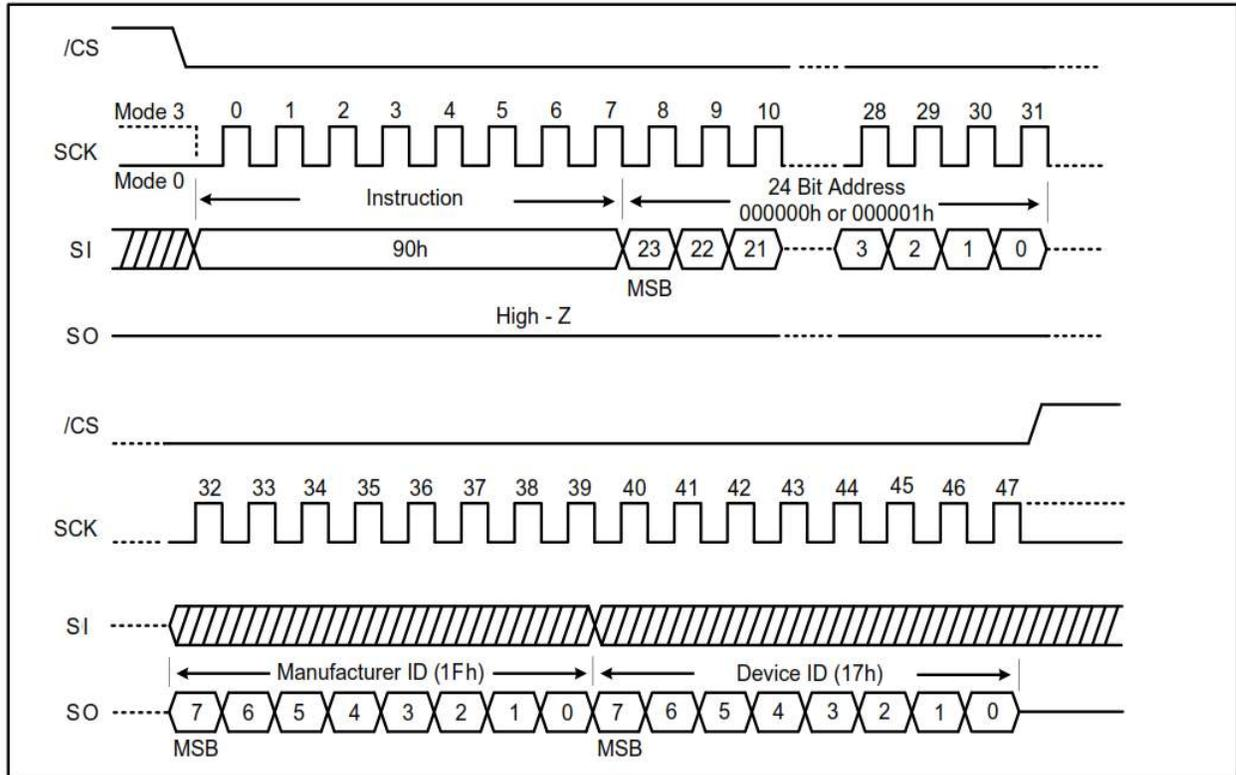
Figure 7-43. Read Manufacturer/ Device ID instruction (QPI Mode)
