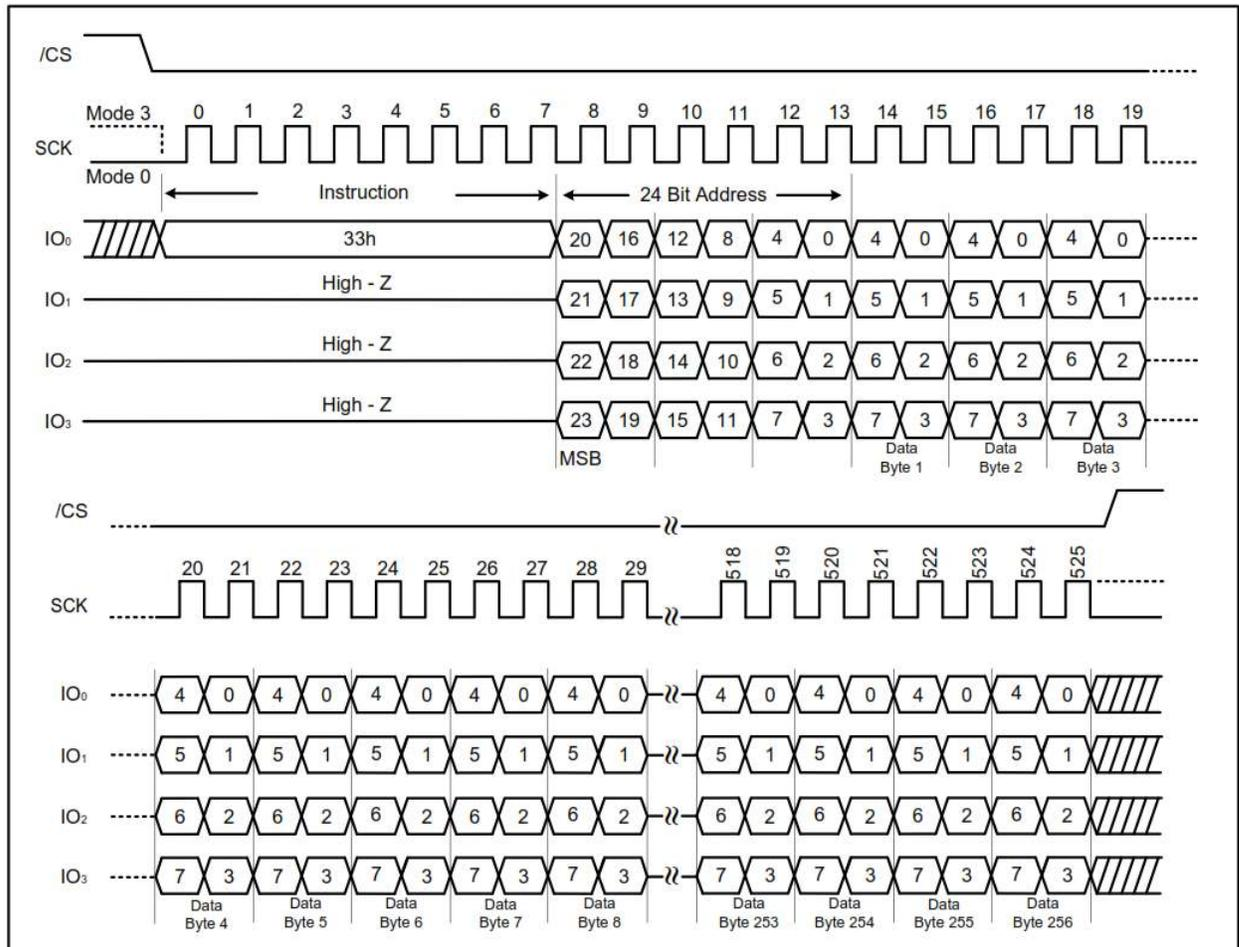
Figure 7-27. Block Erase Instruction (QPI Mode)
