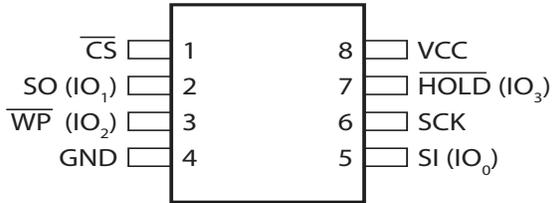
**Figure 1-2. 8-UDFN (Top View)**
