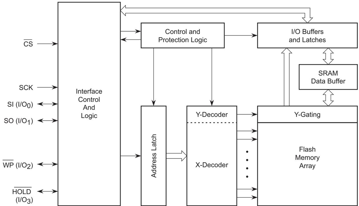
Note: I/O<sub>3-0</sub> pin naming convention is used for Dual-I/O and Quad-I/O commands.
