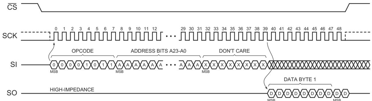
beginning of the array. Deasserting the  $\overline{CS}$  pin terminates the read operation and puts the SO and SI pins into a high-impedance state. The  $\overline{CS}$  pin can be deasserted at any time and does not require that a full byte of data be read.
