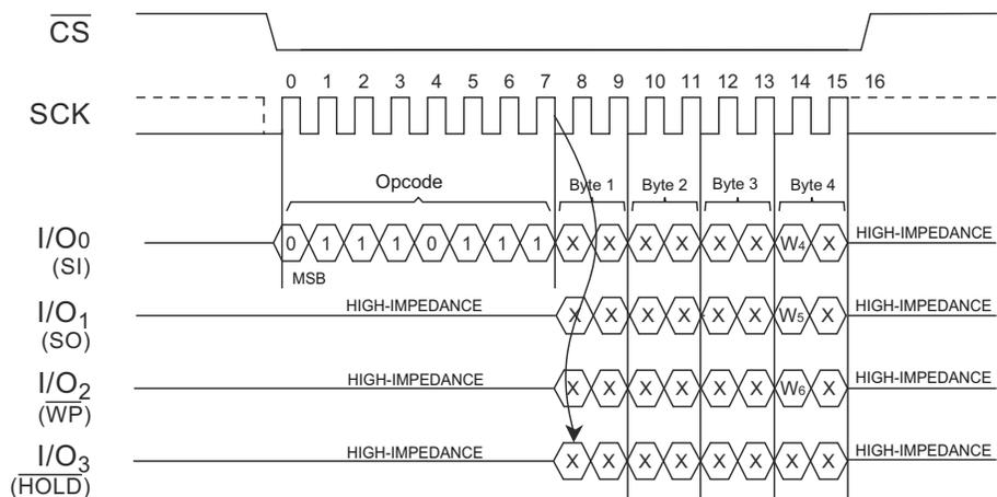
The Set Burst with Wrap instruction sequence is:  $\overline{CS}$  goes low → Send Set Burst with Wrap instruction → Send 24 Dummy bits → Send 8 “Wrap bits” →  $\overline{CS}$  goes high.
