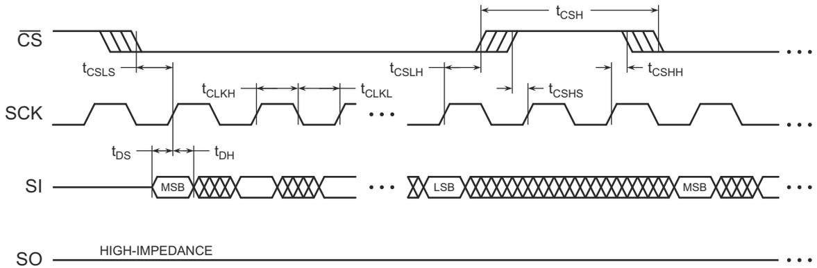
Figure 14-2. Serial Output Timing
