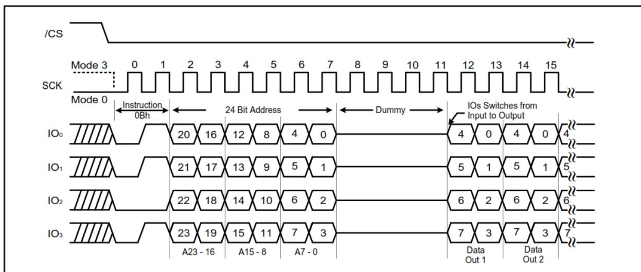
Figure 7-13. Fast Read instruction (QPI Mode, 104MHz)
