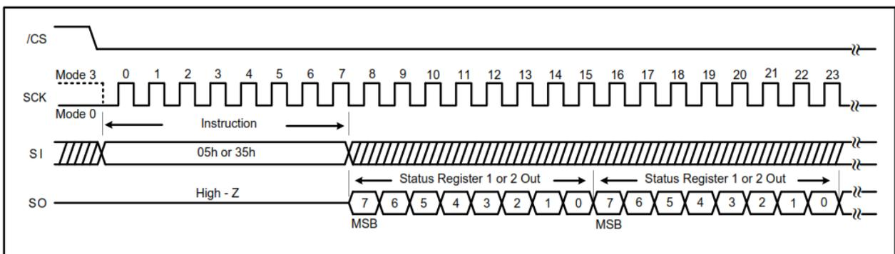
Figure 7-5. Read Status Register Instruction (QPI Mode)
