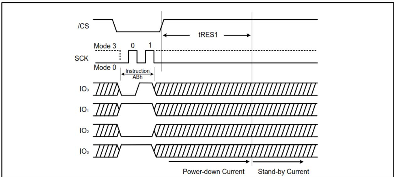
Figure 7-41. Release Power Down / Device ID Instruction (SPI Mode)
