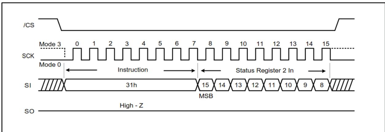
Figure 7-9. Write Status Register-2 Instruction (QPI Mode)
