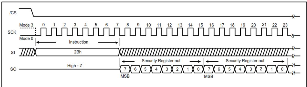
**Figure 7-62. Read Security Register instruction (QPI Mode)**
