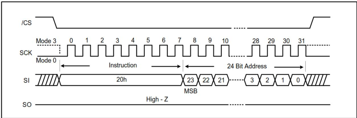
**Figure 7-27. Block Erase Instruction (QPI Mode)**
