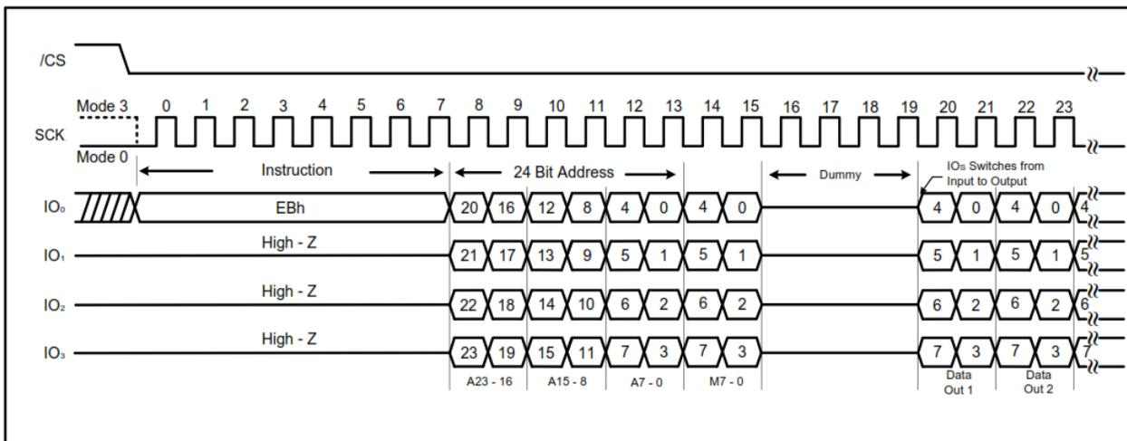
Figure 7-19. Fast Read Quad I/O Instruction (previous M7-0 = Axx, SPI mode)
