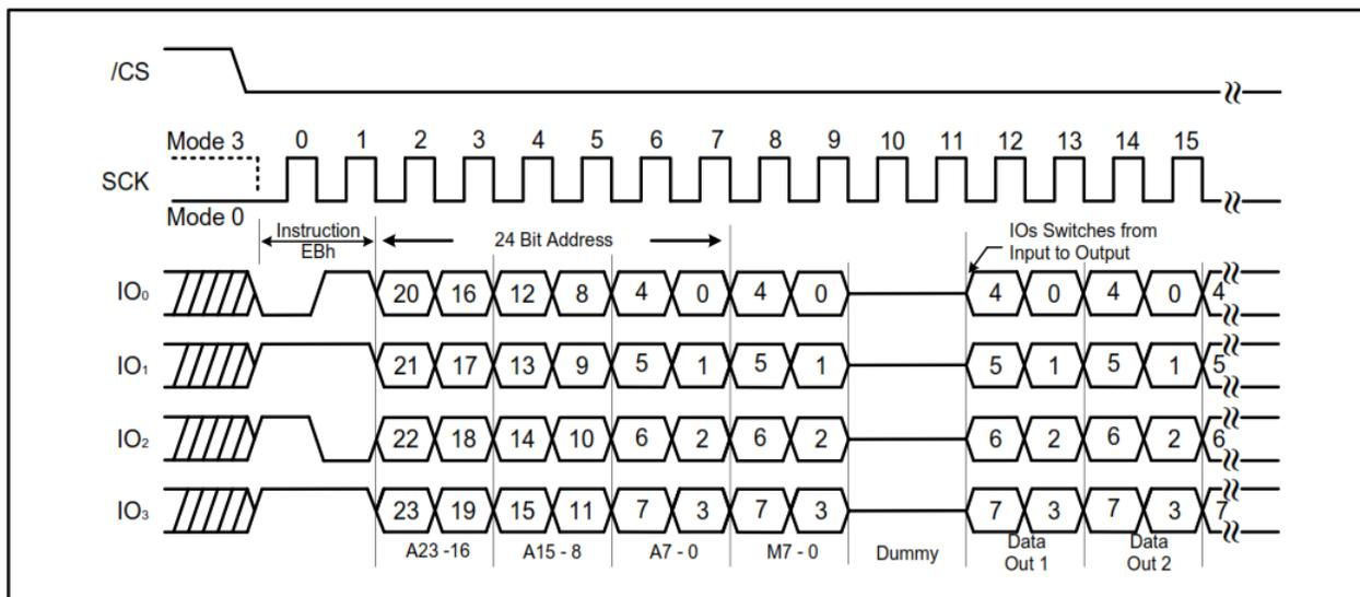
**Figure 7-21. Fast Read Quad I/O Instruction (Initial instruction or previous M7-0 ≠ A<sub>xh</sub>, QPI mode, 104MHz)**
