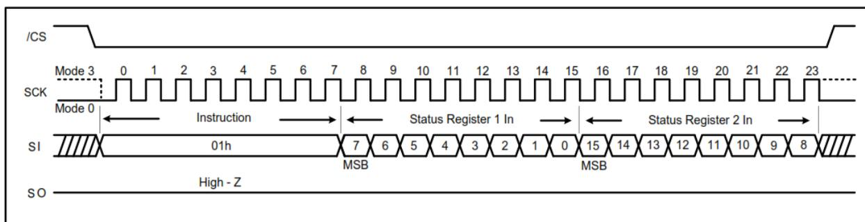
**Figure 7-7. Write Status Register Instruction (QPI Mode)**
