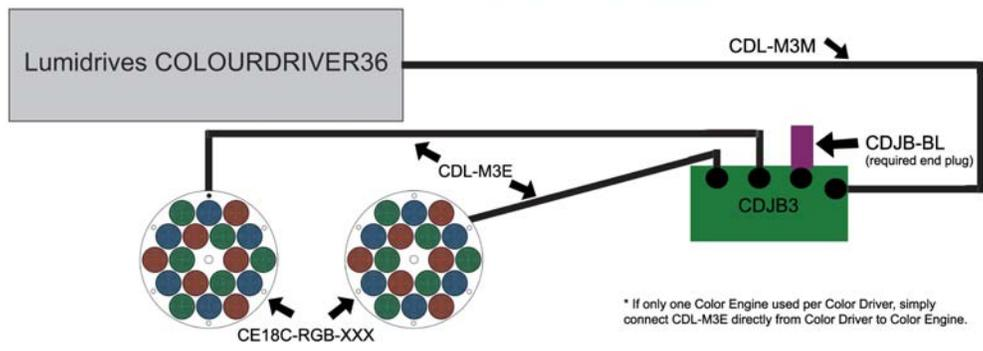
CDL-M3E is equipped with 8 individual colored wires. Each wire to be soldered onto indicated solder pad on color engine. For CE3C-RGB, cut off brown and purple leads.
