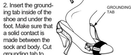
2. Insert the grounding tab inside of the shoe and under the foot. Make sure that a solid contact is made between the sock and body. Cut grounding tab to desired length.
