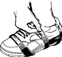
3. Connect the snap-loc fastener together. Adjust elastic strap for comfortable fit. Tuck excess elastic strap behind itself.
