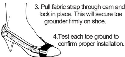
3. Pull fabric strap through cam and lock in place. This will secure toe grounder firmly on shoe.
