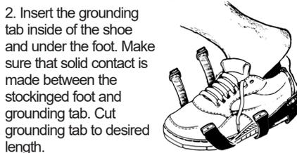
2. Insert the grounding tab inside of the shoe and under the foot. Make sure that solid contact is made between the stockinged foot and grounding tab. Cut grounding tab to desired length.
