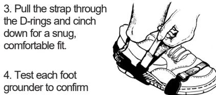
3. Pull the strap through the D-rings and cinch down for a snug, comfortable fit.
