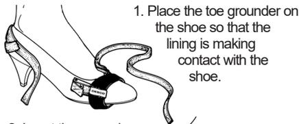
1. Place the toe grounder on the shoe so that the lining is making contact with the shoe.
