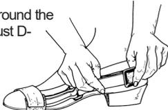
4. Test each toe grounder to confirm proper installation.
