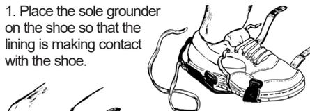
1. Place the sole grounder on the shoe so that the lining is making contact with the shoe.
