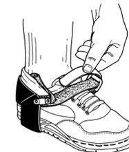
3. Pull the strap through the D-ring and clinch down for a snug, comfortable fit.
