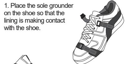
1. Place the sole grounder on the shoe so that the lining is making contact with the shoe.
