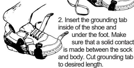
2. Insert the grounding tab inside of the shoe and under the foot. Make sure that a solid contact is made between the sock and body. Cut grounding tab to desired length.
