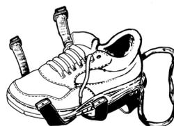
1. Place the full coverage grounder on the shoe so that the lining is making contact with the shoe.
