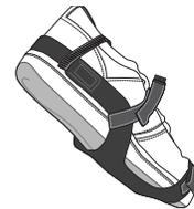
2. Insert the grounding tab inside of the shoe and under the foot. Make sure that a solid contact is made between the sock and body. Cut grounding tab to desired length.
