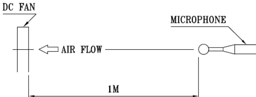
DOISE IS MEASURED AT RATED VOLTAGE IN FREE AIR IN ANECHOIC CHAMBER WITH MICROPHONE AT A DISTANCE OF ONE METER FROM THE FAN INTAKE.
