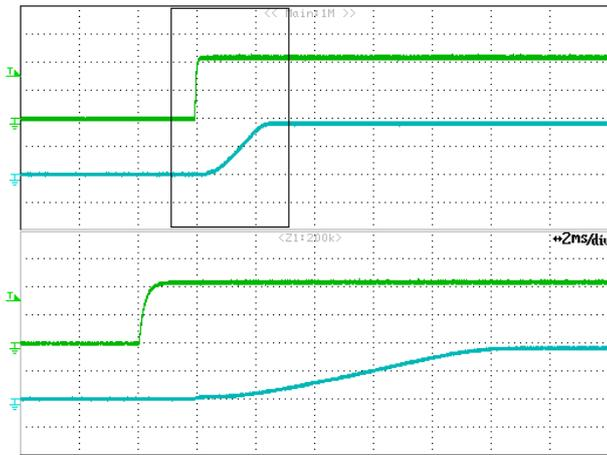
**Figure 12: Remote On/Off Start-up at open load**
