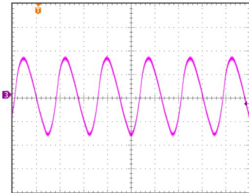
**Figure 19: Input Terminal Ripple Current,  $i_c$ , at max output current, 48Vdc input voltage and 15Vdc output voltage with  $12\mu H$  source impedance and  $33\mu F$  electrolytic capacitor (500 mA/div, 2us/div).**
