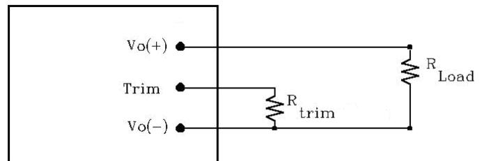
Figure 24: Circuit Configuration for Trim (decrease output voltage)
