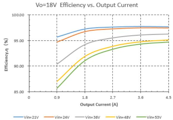
Figure 2: Efficiency vs. Output Current (Vo=18V)
