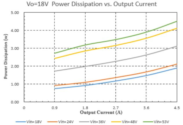
Figure 6: Power Dissipation vs. Output Current( $V_o=18V$ )
