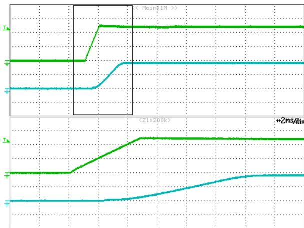
**Figure 14: Input Voltage Start-up at open load**
