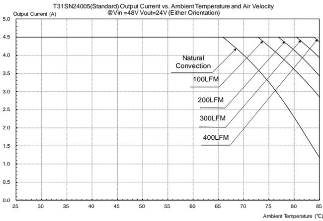
**Figure 30:** Output current vs. ambient temperature and air velocity @ $V_{in}=48V$ ,  $V_{out}=24V$  (Either Orientation, Open Frame)
