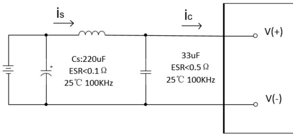
**Figure 18: Test Setup Diagram for Input Ripple Current**
