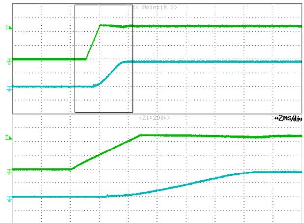
**Figure 15: Input Voltage Start-up at full load**
