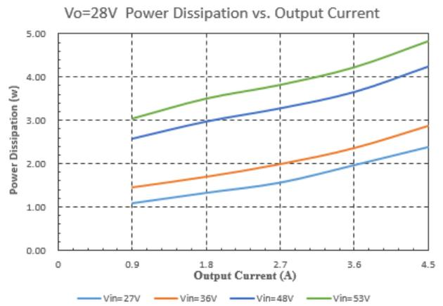
Figure 8: Power Dissipation vs. Output Current( $V_o=28V$ )
