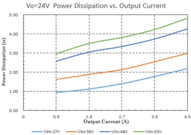
Figure 7: Power Dissipation vs. Output Current( $V_o=24V$ )
