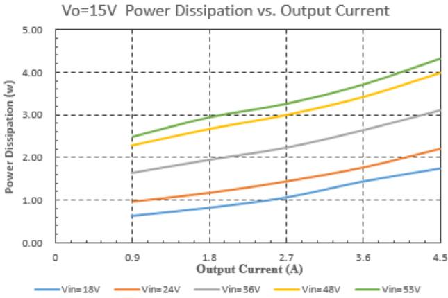
Figure 5: Power Dissipation vs. Output Current( $V_o=15V$ )
