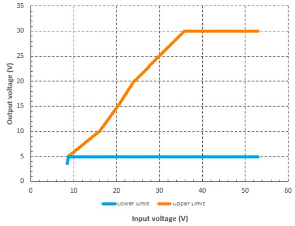
**Figure 10: Output Voltage versus Input Voltage Operating Range**
