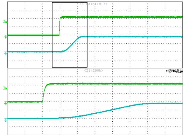
**Figure 13: Remote On/Off Start-up at full load**
