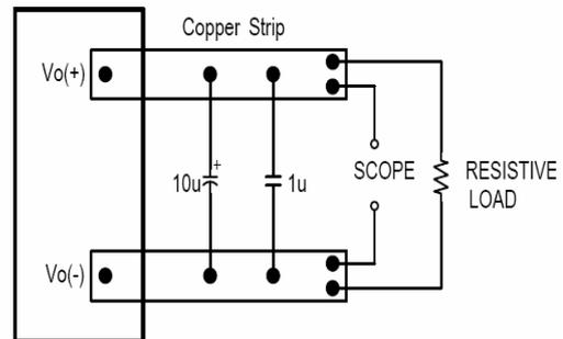
Output voltage ripple test setup.
