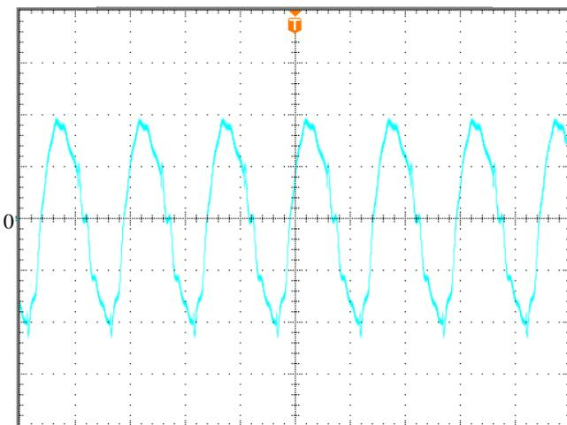
Output voltage ripple at nominal input voltage and max load current (30mV/div, 2us/div)
