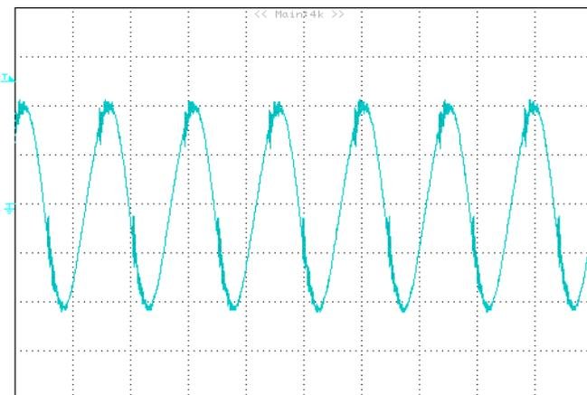
Output voltage ripple at nominal input voltage and max load current (20mV/div, 2us/div)
