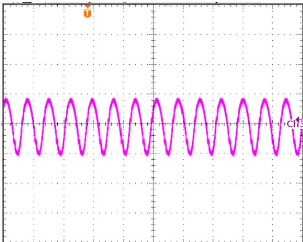
Input Terminal Ripple Current,  $i_c$ , at full rated output current and nominal input voltage with  $12\mu\text{H}$  source impedance and  $100\mu\text{F}$  electrolytic capacitor (250 mA/div, 4us/div).
