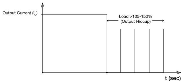
It is not recommended to prolong the duration of  $I_o$  when it is <105% but >100%, since it may cause damage to the PSU.
