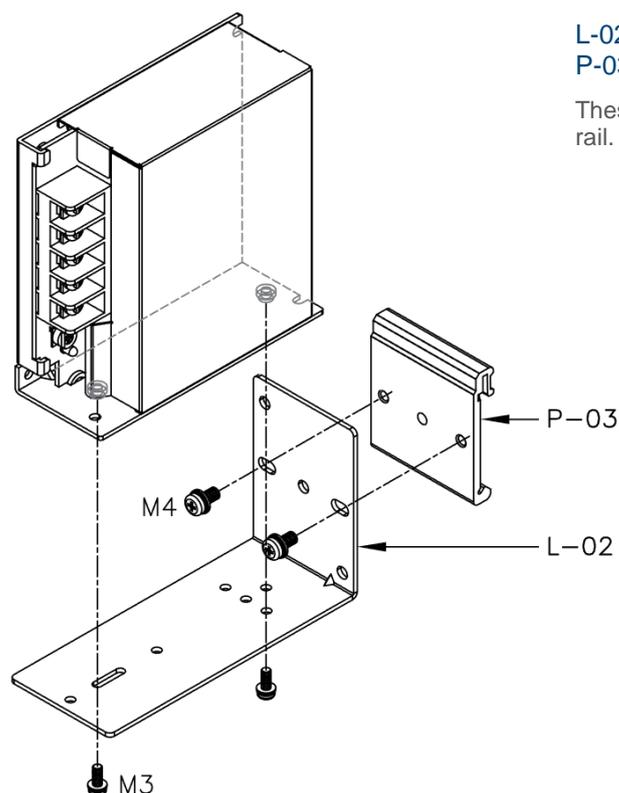
These accessories are used to mount the panel mount power supply onto a DIN rail.
