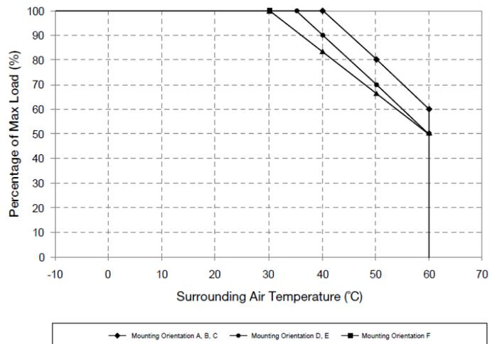
Fig.1.2 De-rating for Mounting Orientation A, B, C
