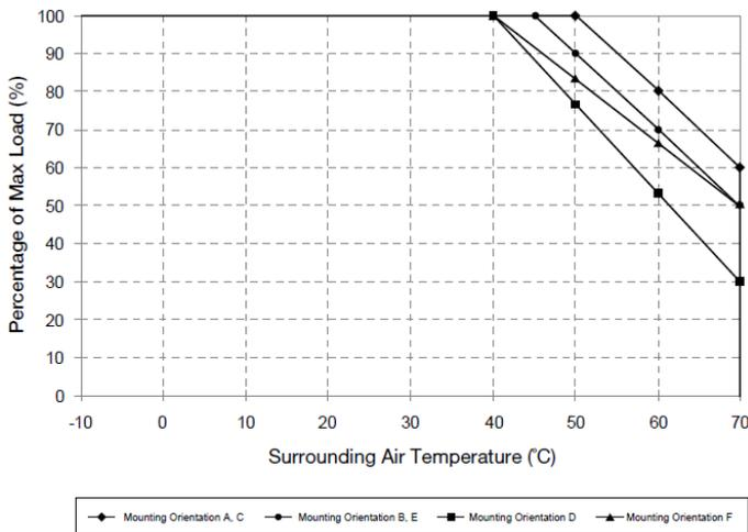
Fig.1.1 De-rating for Mounting Orientation A, C
