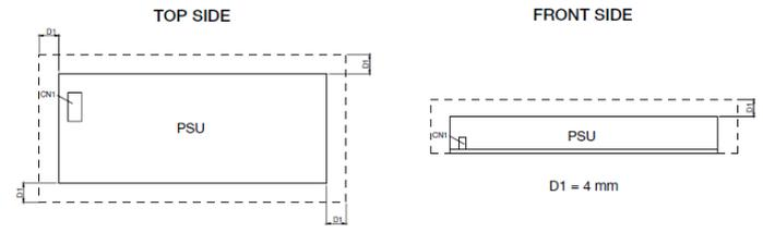
For safety reasons, please ensure the mounted device is kept at  $\geq 4$  mm safety distance at all sides from other components and equipments. **Please insert an insulation sheet between the system and product, if the safety distance is less than 4mm.**
