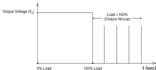
Additionally, if the  $I_o$  is  $<105\%$  but  $>100\%$  for a prolonged period of time (depending on the load), the Over Temperature Protection (OTP) will be activated due to high temperature on critical components. The power supply will then go into latch mode until the fault is removed and the mains is reapplied.
