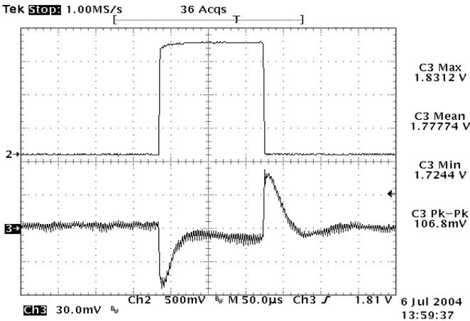
Figure 21: Typical transient response to step load change at 10A/μs from 50% to 75% and 75% to 50% of I<sub>o</sub>, max at 12V<sub>in</sub>, 1.8V out
