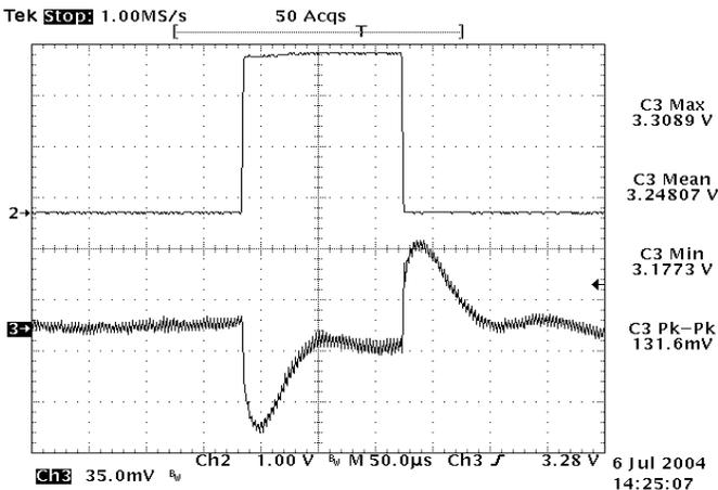
Figure 23: Typical transient response to step load change at 10A/μs from 50% to 75% and 75% to 50% of I<sub>o</sub>, max at 12V<sub>in</sub>, 3.3V out
