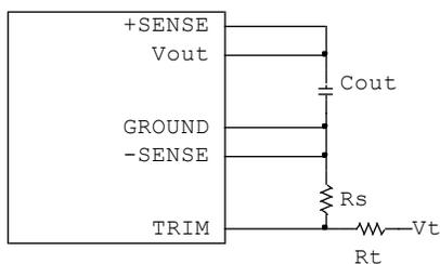
Figure 33: Output voltage trim with voltage source
