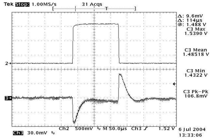
Figure 20: Typical transient response to step load change at 10A/μs from 50% to 75% and 75% to 50% of I<sub>o</sub>, max at 12V<sub>in</sub>, 1.5V out
