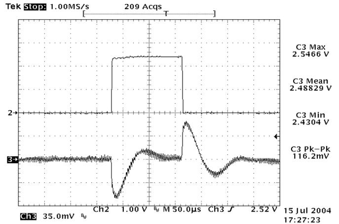
Figure 22: Typical transient response to step load change at 10A/μs from 50% to 75% and 75% to 50% of I<sub>o</sub>, max at 12V<sub>in</sub>, 2.5V out
