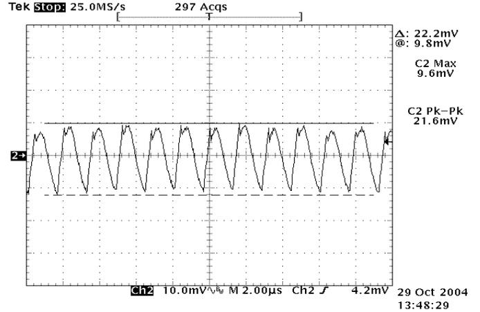
Figure 8: Output ripple & noise at 12Vin, 0.9V/40A out
