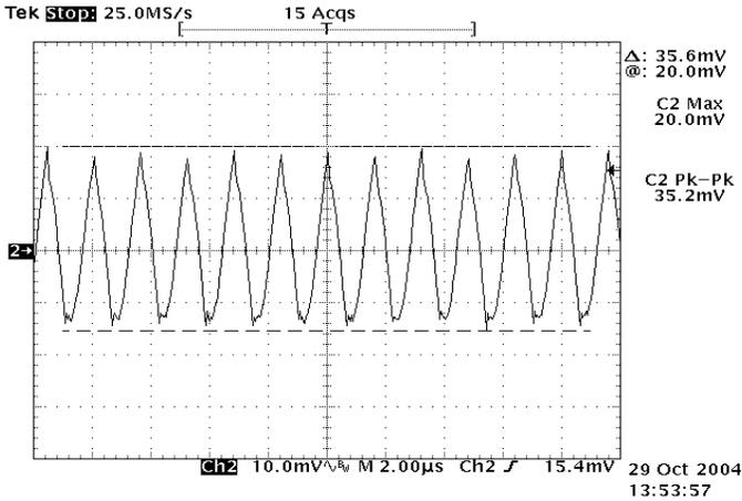
Figure 13: Output ripple & noise at 12Vin, 3.3V/40A out
