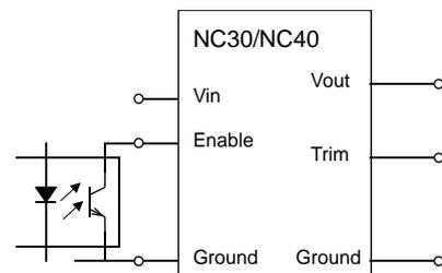
Figure 28: Enable input drive circuit example with isolation.
