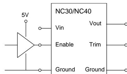
Figure 27: Enable input drive circuit using logic gate.
