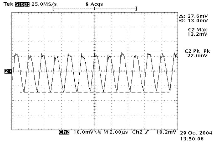
Figure 10: Output ripple & noise at 12Vin, 1.5V/40A out
