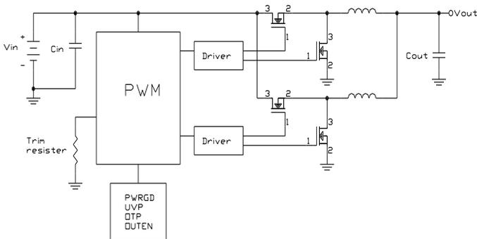
Figure 25: Block Diagram
