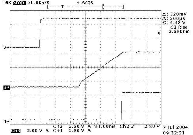
Figure 18: Turn on delay time Remote On/Off, 5V/40A out
