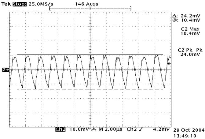
Figure 9: Output ripple & noise at 12Vin, 1.2V/40A out
