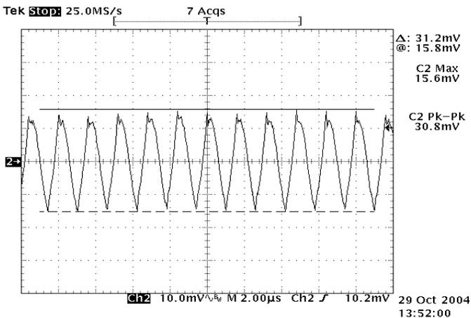
Figure 11: Output ripple & noise at 12Vin, 1.8V/40A out
