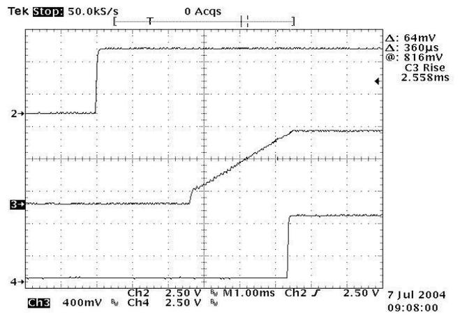
Figure 16: Turn on delay time Remote On/Off, 0.9V/40A out
