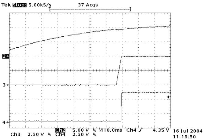
Figure 17: Turn on delay time at 12Vin, 5V/40A out
