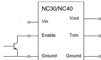
Figure 26: Enable Input drive circuit for NC series
