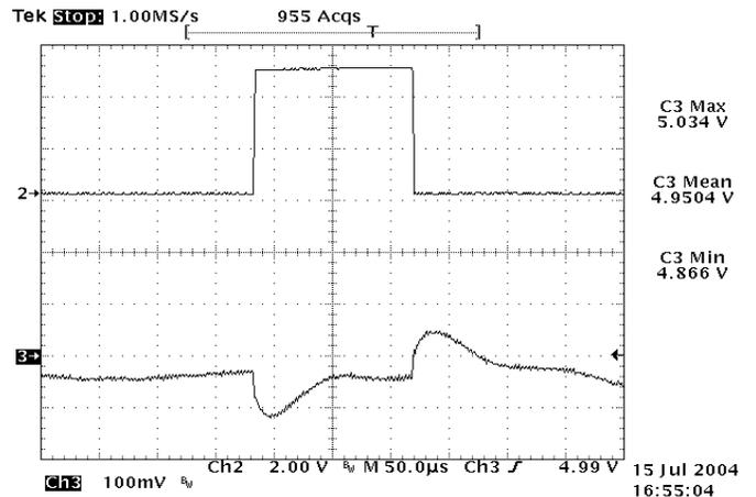
Figure 24: Typical transient response to step load change at 10A/μs from 50% to 75% and 75% to 50% of I<sub>o</sub>, max at 12V<sub>in</sub>, 5.0V out
