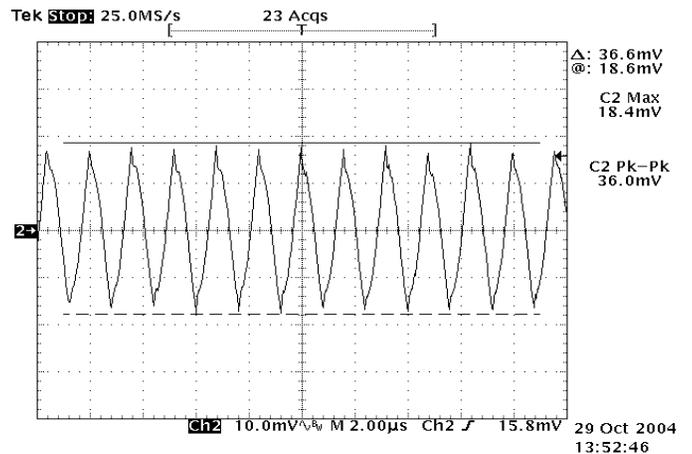
Figure 12: Output ripple & noise at 12Vin, 2.5V/40A out
