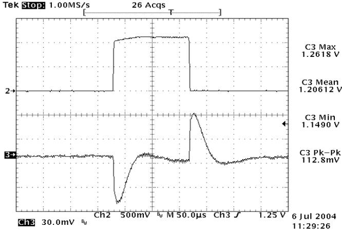
Figure 19: Typical transient response to step load change at 10A/μs from 50% to 75% and 75% to 50% of I<sub>o</sub>, max at 12V<sub>in</sub>, 1.2V out
