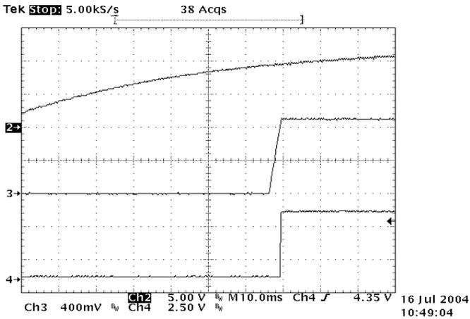
Figure 15: Turn on delay time at 12Vin, 0.9V/40A out
