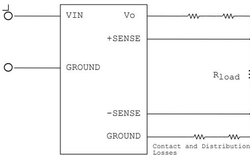
**Figure 29:** Circuit configuration for remote sense
