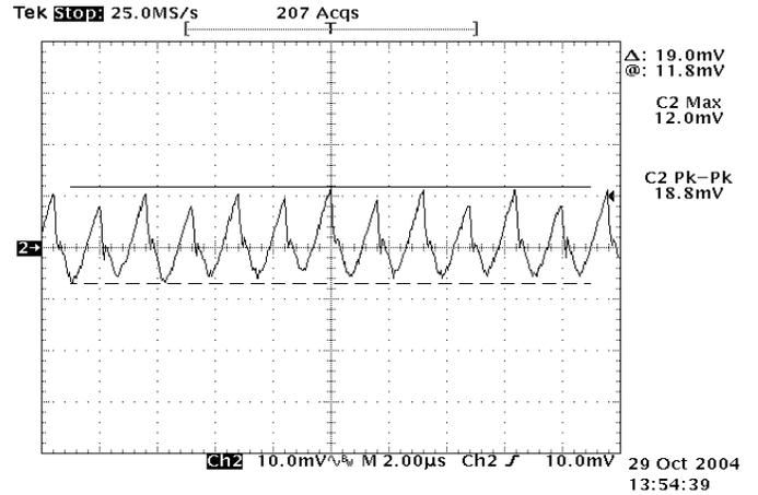
Figure 14: Output ripple & noise at 12Vin, 5V/40A out
