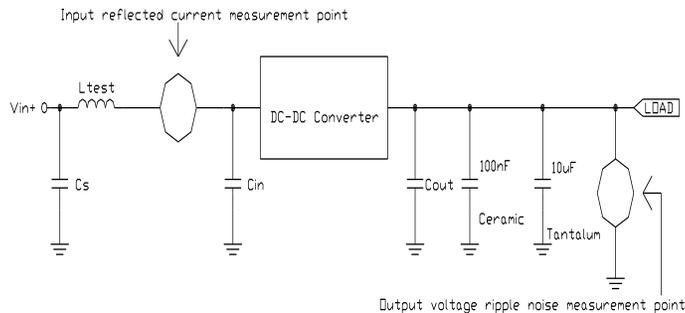
$$C_s = 270\mu F * 1 \quad L_{test} = 1.4\mu H \quad C_{in} = 270\mu F * 2 \quad C_{out} = 680\mu F * 3$$
