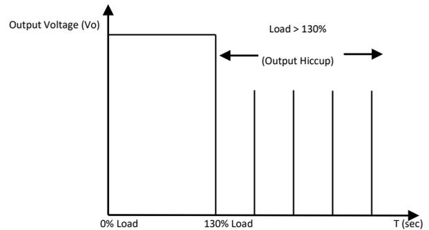
Additionally, if the  $I_o$  is  $< 130\%$  but  $> 110\%$  for a prolonged period of time (depending on the load), the Over Temperature Protection (OTP) will be activated due to high temperature on critical components. The power supply will then go into hiccup mode until the fault is removed; and, the input voltage is removed, then reapplied.
