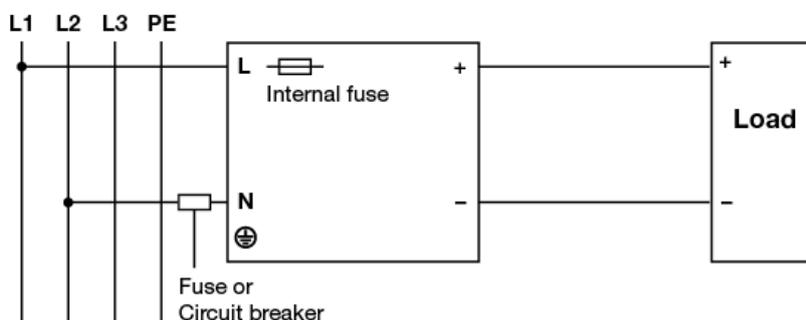
Fig. 7 2 of 3 Phase System Input Operation Connection Diagram
