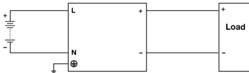
Fig. 6 DC Input Operation Connection Diagram
