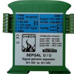
SEPGAL U / U separator is used to provide galvanic isolation between two circuits of standard analog signals, voltage type 0-10V or 1-10V.
