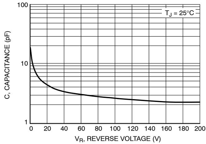
**Figure 3. Typical Capacitance**
