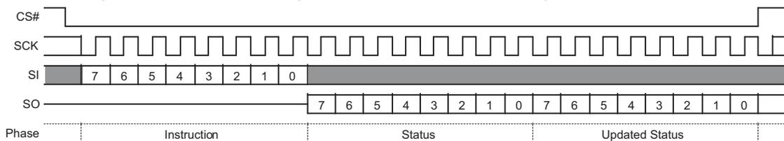
**Figure 31. Read Status Register-3 Command Sequence Diagram for 33h — S25FL132K / S25FL164K**
