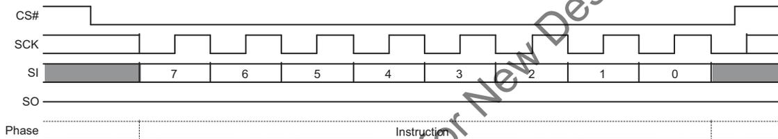
**10.1.3 Write Enable for Volatile Status Register (50h)**
