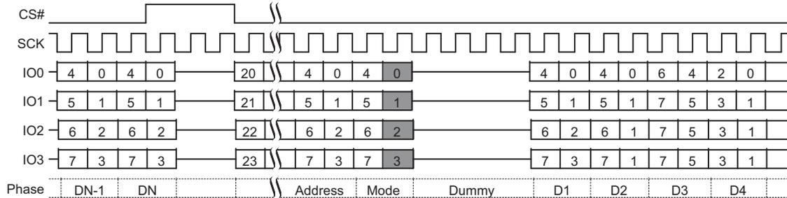
**Fast Read Quad I/O with “16 / 32 / 64-Byte Wrap Around”**
