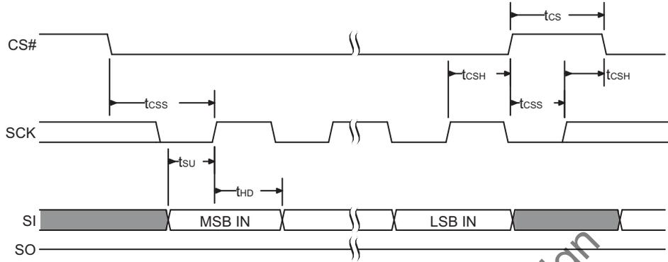
Figure 22. PI Single Bit Output Timing
