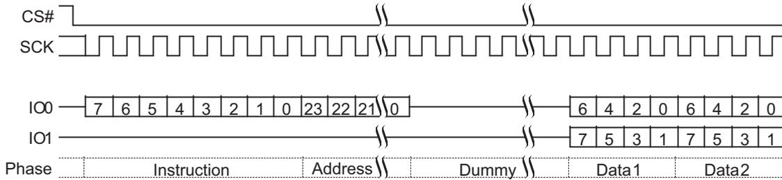
Figure 11. Quad Output Command without Latency
