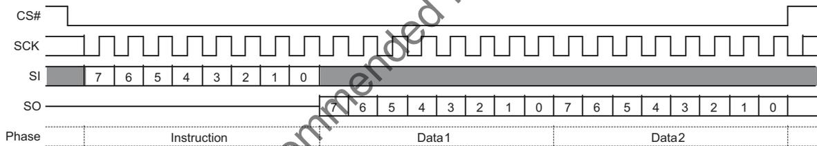
Figure 8. Single Bit Wide I/O Command without Latency
