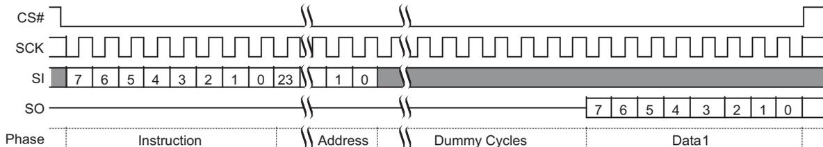
Figure 10. Dual Output Command
