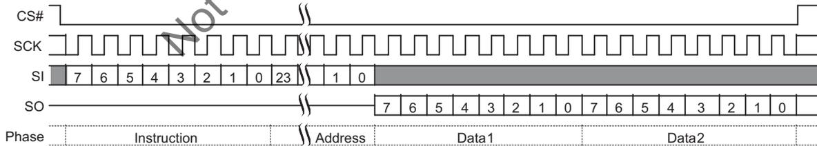
Figure 9. Single Bit Wide I/O Command with Latency
