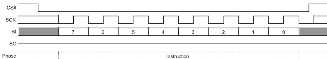
Figure 55. Read Electronic Signature (RES ABh) Command Sequence
