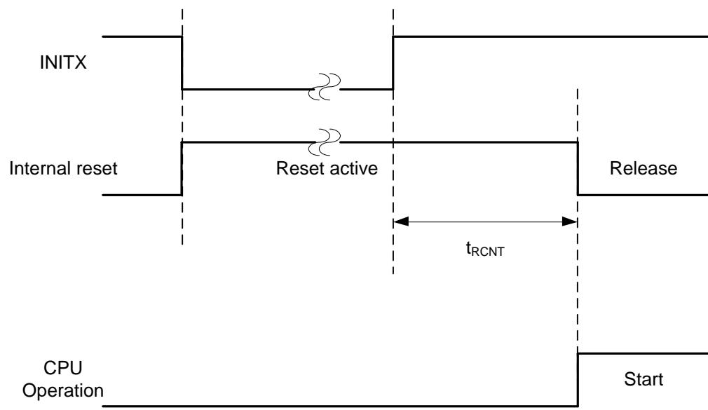
**Operation example of return from low power consumption mode (by internal resource reset\*)**
