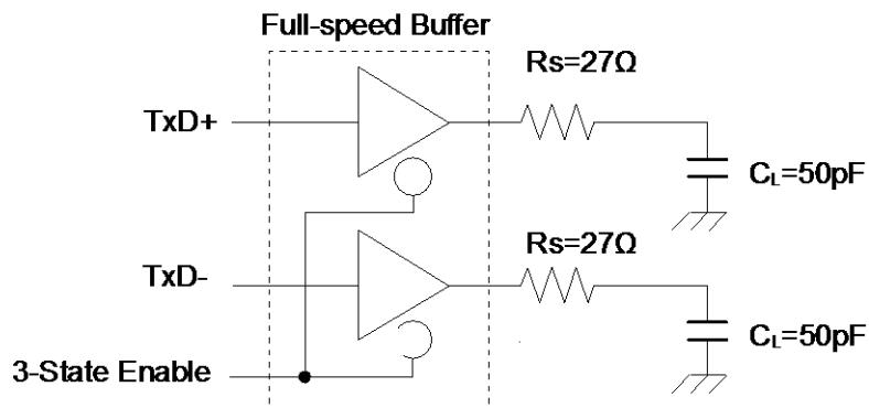
\*6: USB Full-speed connection is performed via twist pair cable shield with  $90\ \Omega \pm 15\%$  characteristic impedance (Differential Mode).
