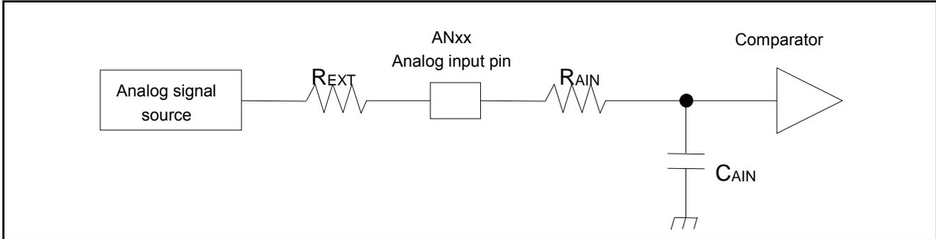
$$\text{(Equation 1) } t_s \geq (R_{AIN} + R_{EXT}) \times C_{AIN} \times 9$$
