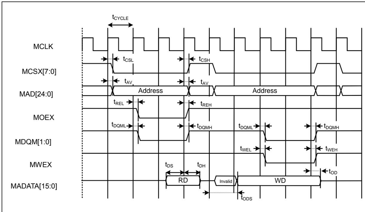
**Multiplexed Bus Access Asynchronous SRAM Mode**
