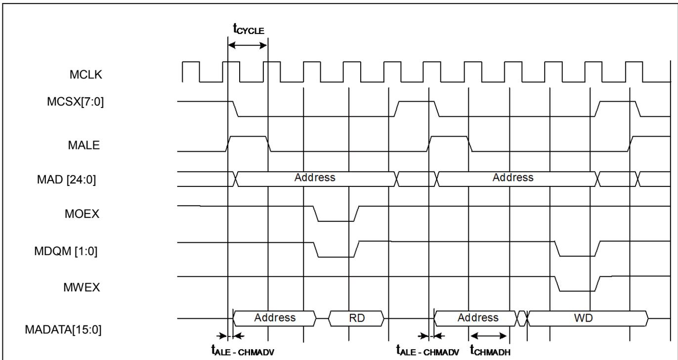
**Multiplexed Bus Access Synchronous SRAM Mode**
