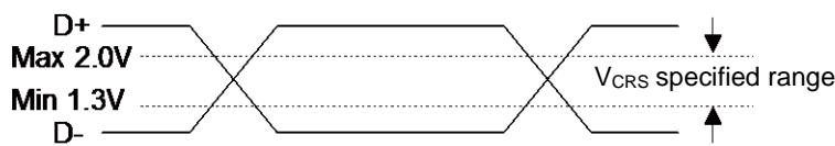
\*5: They indicate rising time (Trise) and falling time (Tfall) of the full-speed differential data signal. They are defined by the time between 10% and 90% of the output signal voltage. For full-speed buffer, Tr/Tf ratio is regulated as within  $\pm 10\%$  to minimize RFI emission.
