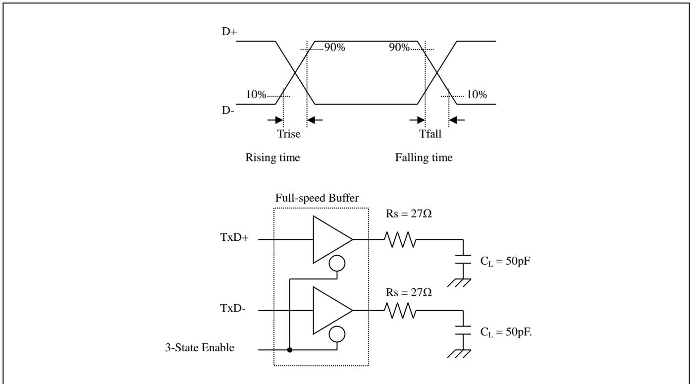
\*6: USB Full-speed connection is performed via twist pair cable shield with  $90 \Omega \pm 15\%$  characteristic impedance (Differential Mode).
