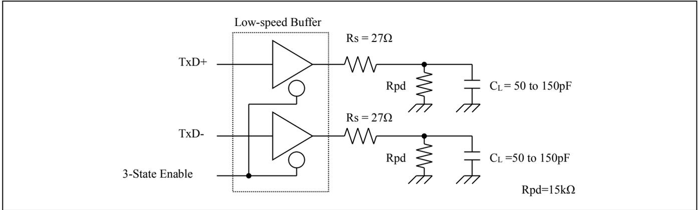
**Low-Speed Load (Downstream Port Load) - Reference 2**
