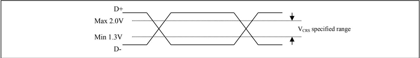
\*5: They indicate rise time ( $T_{rise}$ ) and fall time ( $T_{fall}$ ) of the full-speed differential data signal. They are defined by the time between 10% and 90% of the output signal voltage. For full-speed buffer,  $T_r/T_f$  ratio is regulated as within  $\pm 10\%$  to minimize RFI emission.
