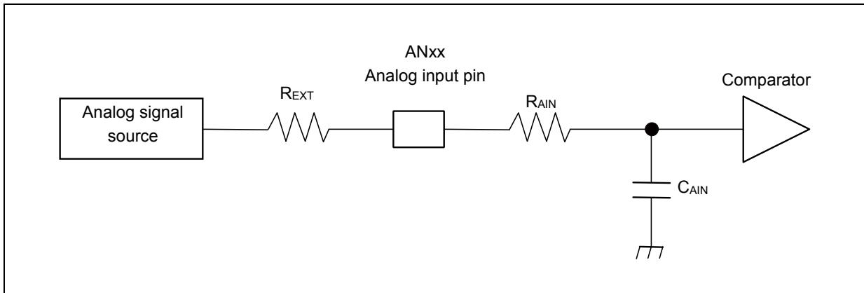
(Equation 1)  $t_s \geq (R_{AIN} + R_{EXT}) \times C_{AIN} \times 9$
