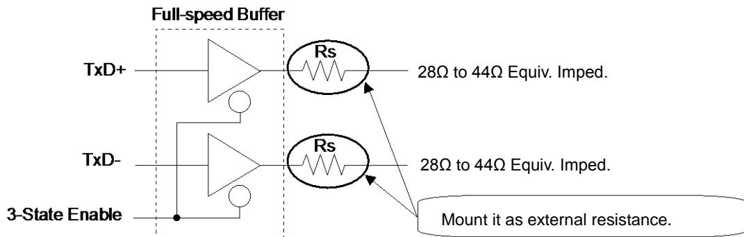
Rs series resistor  $25\Omega$  to  $30\Omega$
