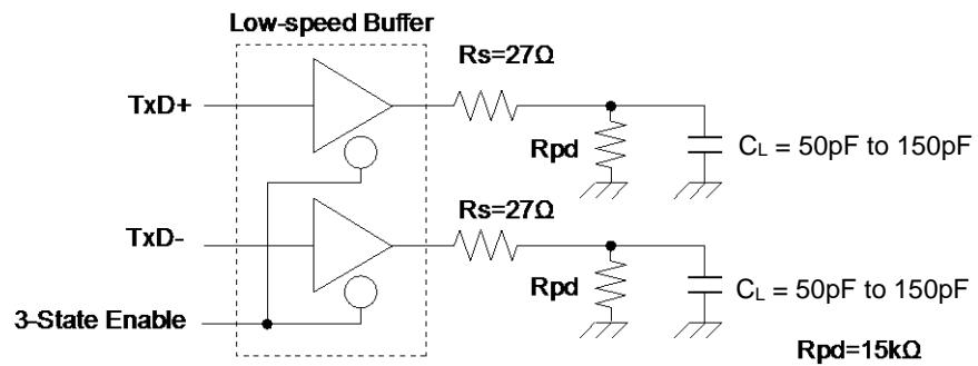
**Low-Speed Load (Downstream Port Load) - Reference 2**
