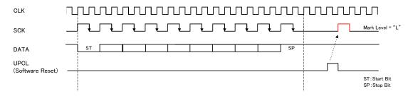
The connected slave device may consider this pulse on SCK line as a serial clock.
