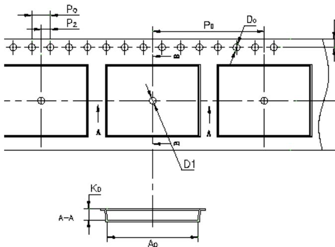
Figure 18 details the orientation of the CYBLE-0130XX-00 in the tape as well as the direction for unreeling.
