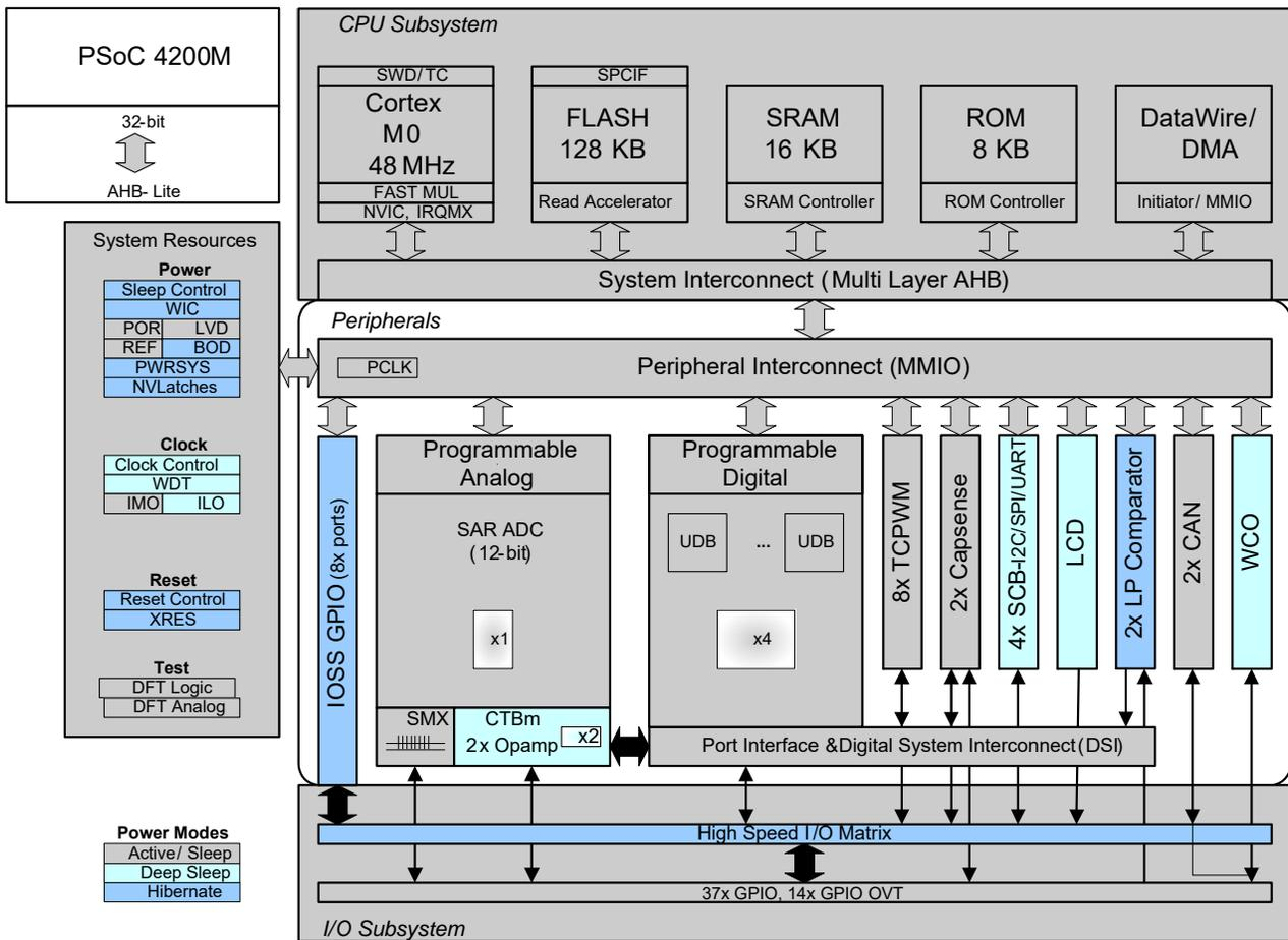
The PSoC 4200M devices include extensive support for programming, testing, debugging, and tracing both hardware and firmware.
