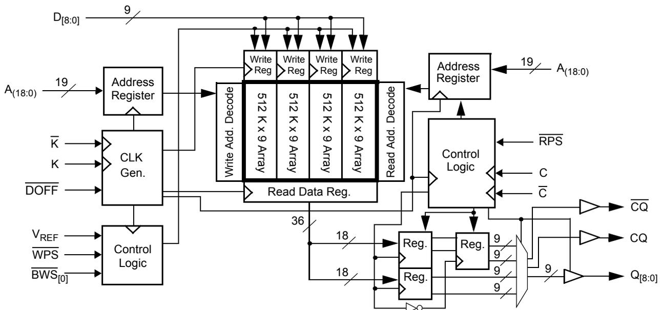
Logic Block Diagram – CY7C1313KV18
