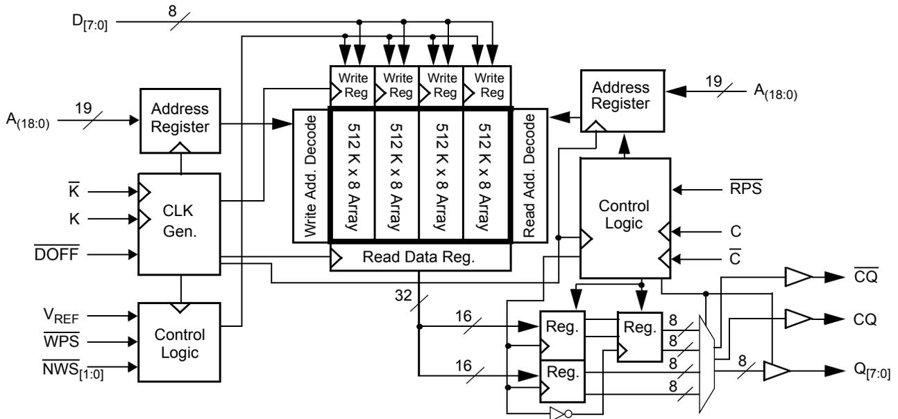
Logic Block Diagram – CY7C1911KV18
