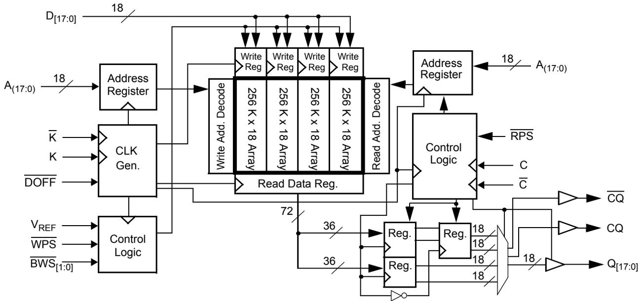
Logic Block Diagram – CY7C1315KV18
