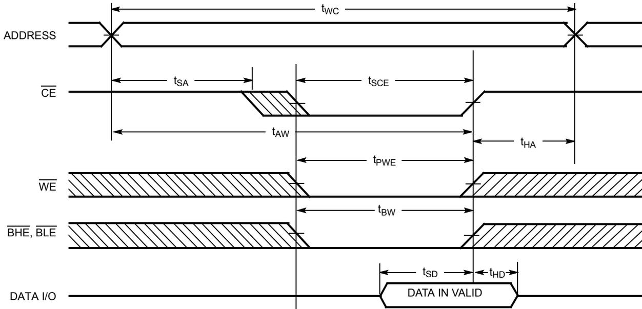
Figure 9. Write Cycle No. 2 ( $\overline{\text{WE}}$  Controlled,  $\overline{\text{OE}}$  LOW) [24, 25, 26]
