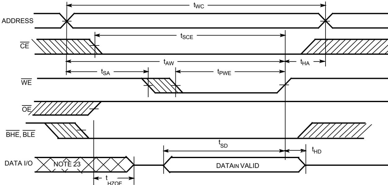
Write Cycle No. 4 ( $\overline{WE}$  Controlled,  $\overline{OE}$  LOW)
