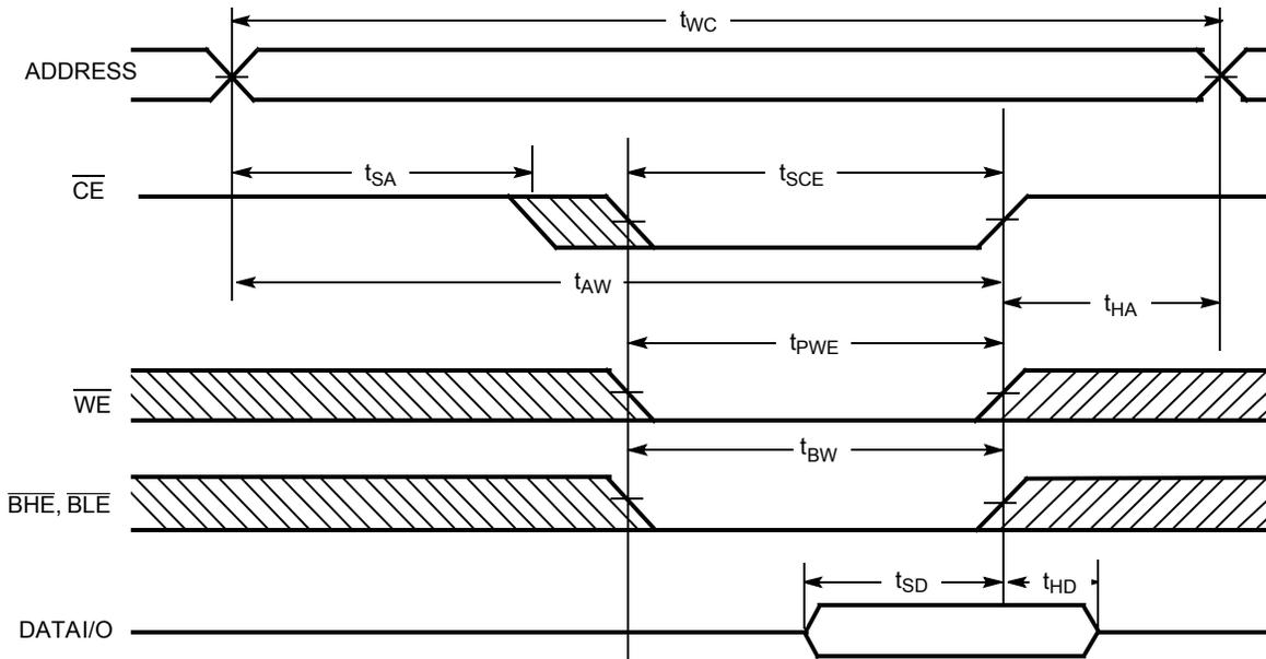
Write Cycle No. 2 ( $\overline{\text{BLE}}$  or  $\overline{\text{BHE}}$  Controlled)
