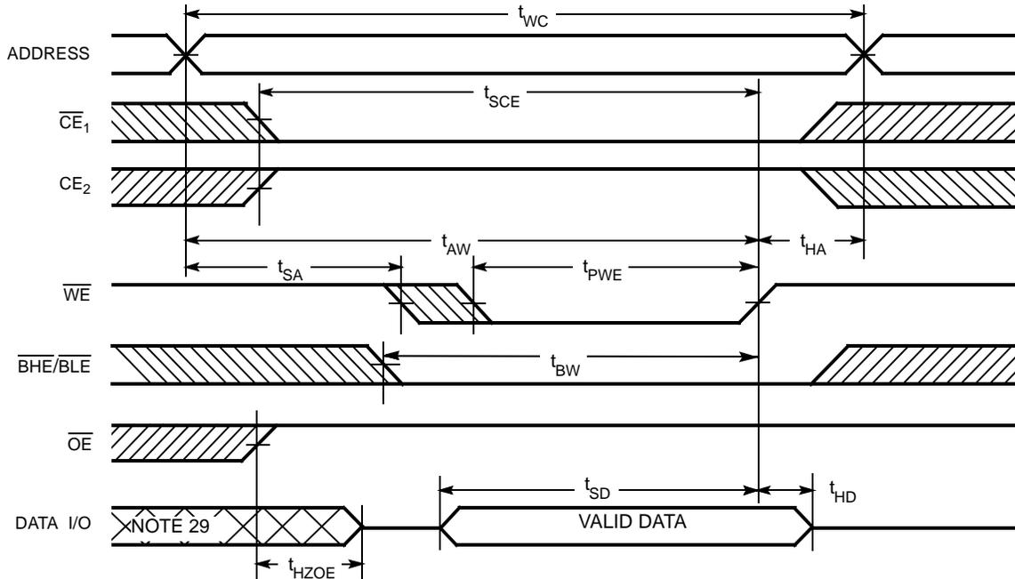
Figure 8. Write Cycle 2 ( $\overline{CE_1}$  or  $\overline{CE_2}$  Controlled) [26, 27, 28, 29]
