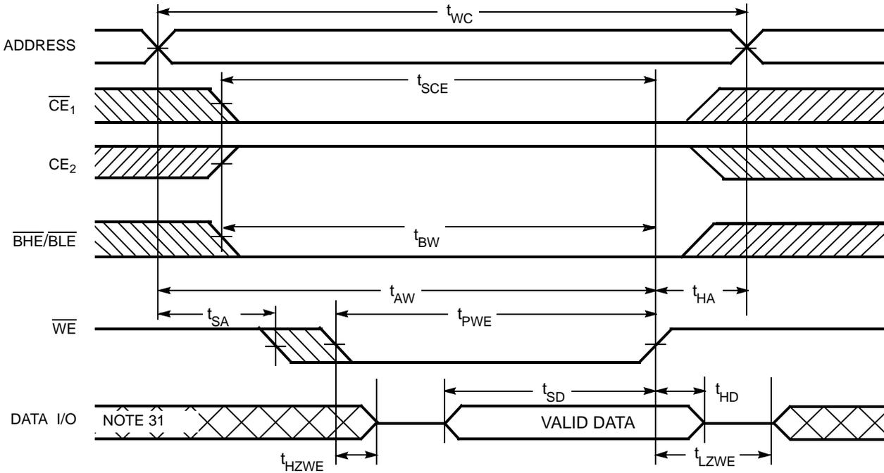
Figure 10. Write Cycle 4 ( $\overline{BHE}/\overline{BLE}$  Controlled,  $\overline{OE}$  LOW) [30, 32]
