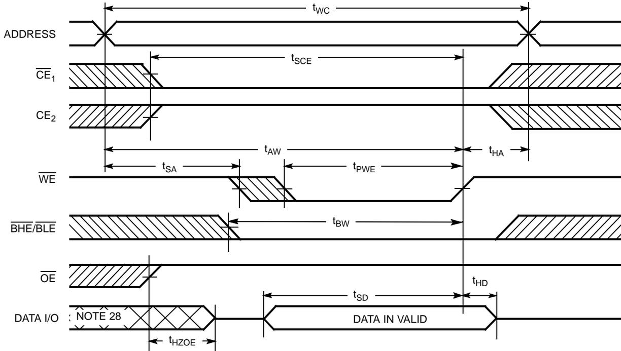
Figure 7. Write Cycle No. 2 ( $\overline{CE}_1$  or  $\overline{CE}_2$  Controlled) [25, 26, 27]
