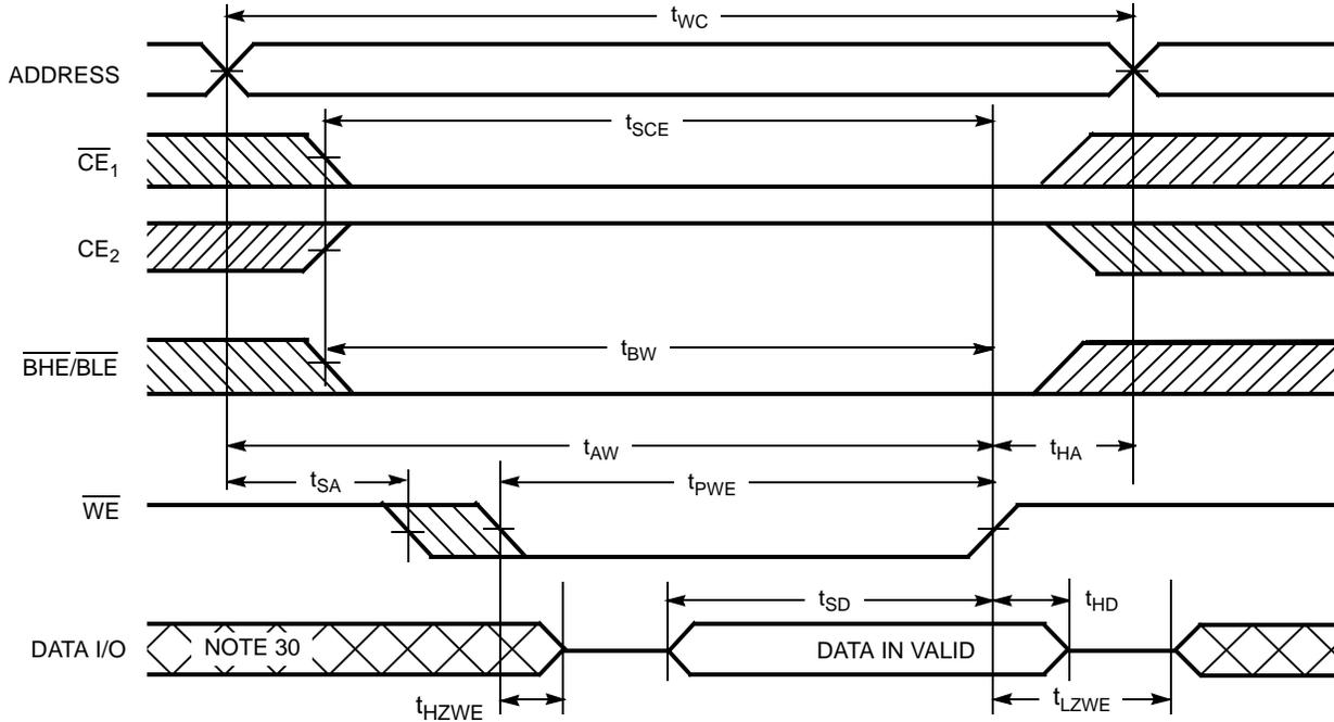
Figure 9. Write Cycle No. 4 ( $\overline{BHE}/\overline{BLE}$  Controlled) [29]
