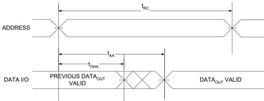
Figure 7. Read Cycle No. 2 ( $\overline{\text{OE}}$  Controlled)<sup>[26, 27, 28]</sup>
