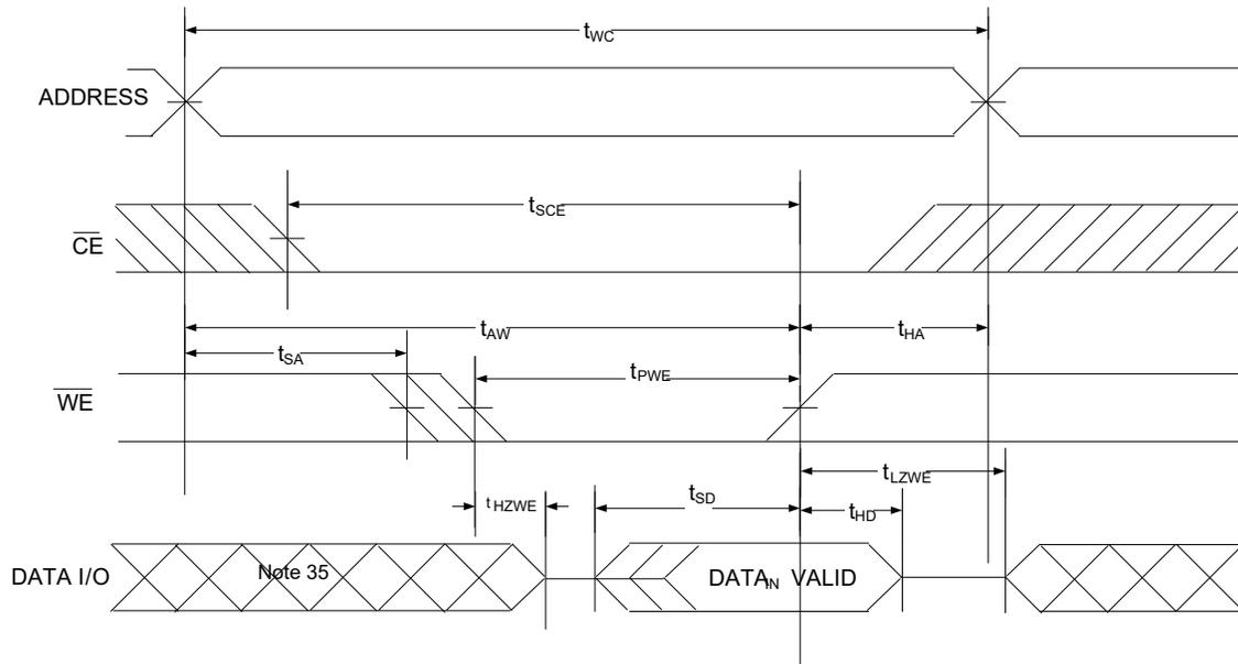
Figure 10. Write Cycle No. 3 ( $\overline{CE}$  Controlled)<sup>[32, 33, 34]</sup>
