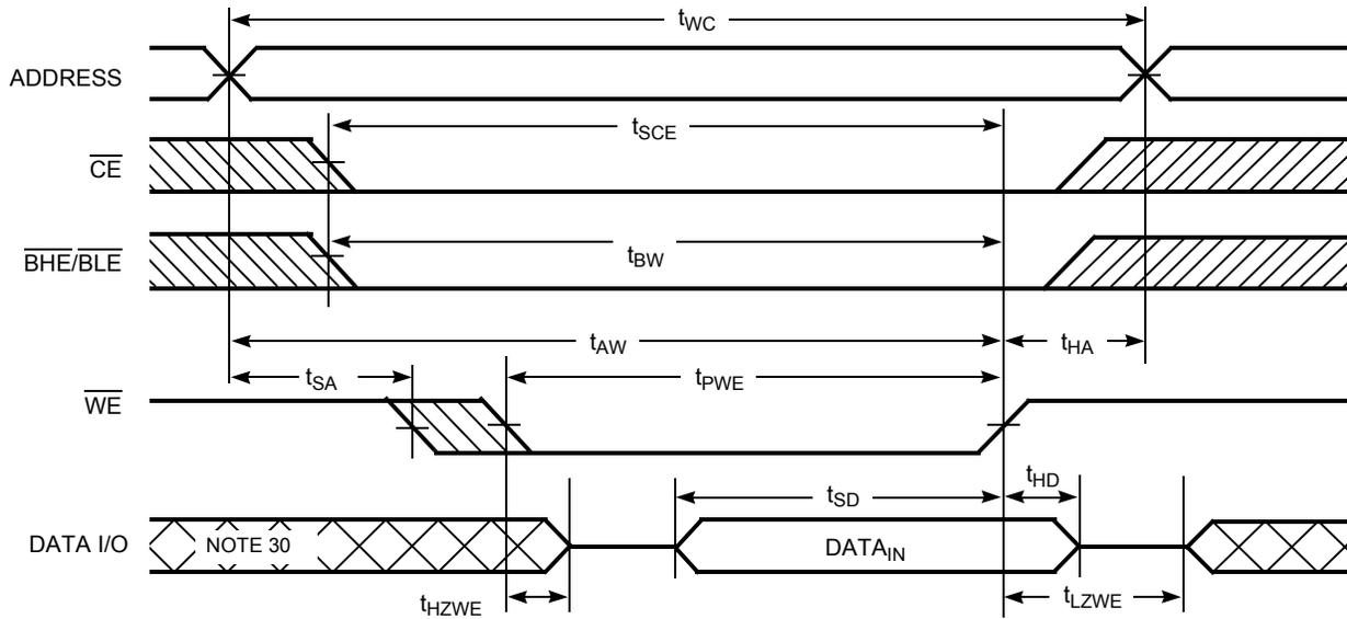
**Figure 9. Write Cycle 4:  $\overline{BHE/BLE}$  Controlled,  $\overline{OE}$  LOW [28]**
