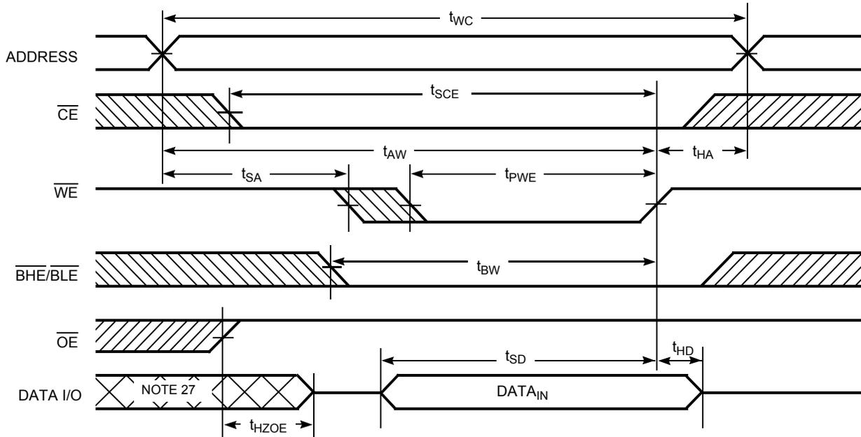
Figure 7. Write Cycle 2:  $\overline{CE}$  Controlled [24, 25, 26]
