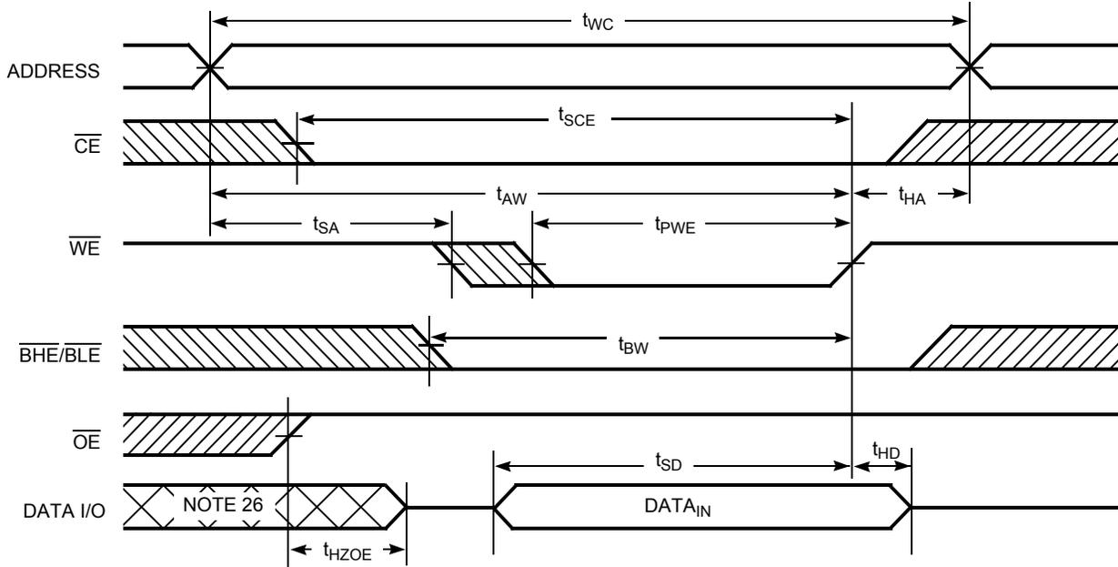
Figure 8. Write Cycle 2:  $\overline{CE}$  Controlled [23, 24, 25]
