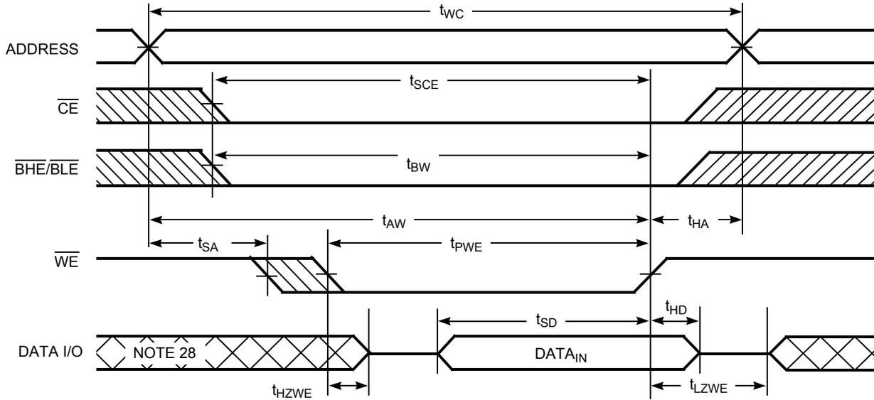
Figure 10. Write Cycle 4:  $\overline{BHE}/\overline{BLE}$  Controlled,  $\overline{OE}$  LOW <sup>[27]</sup>
