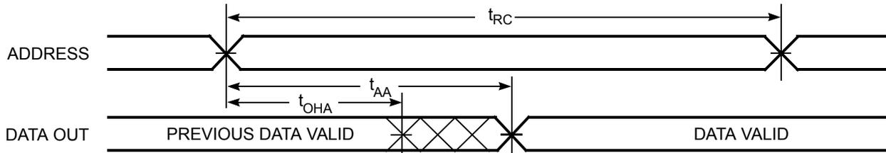
Figure 6. Read Cycle No. 2:  $\overline{OE}$  Controlled [21, 22]
