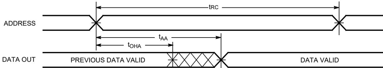
Figure 7. Read Cycle No. 2 ( $\overline{OE}$  Controlled) [22, 23, 24]
