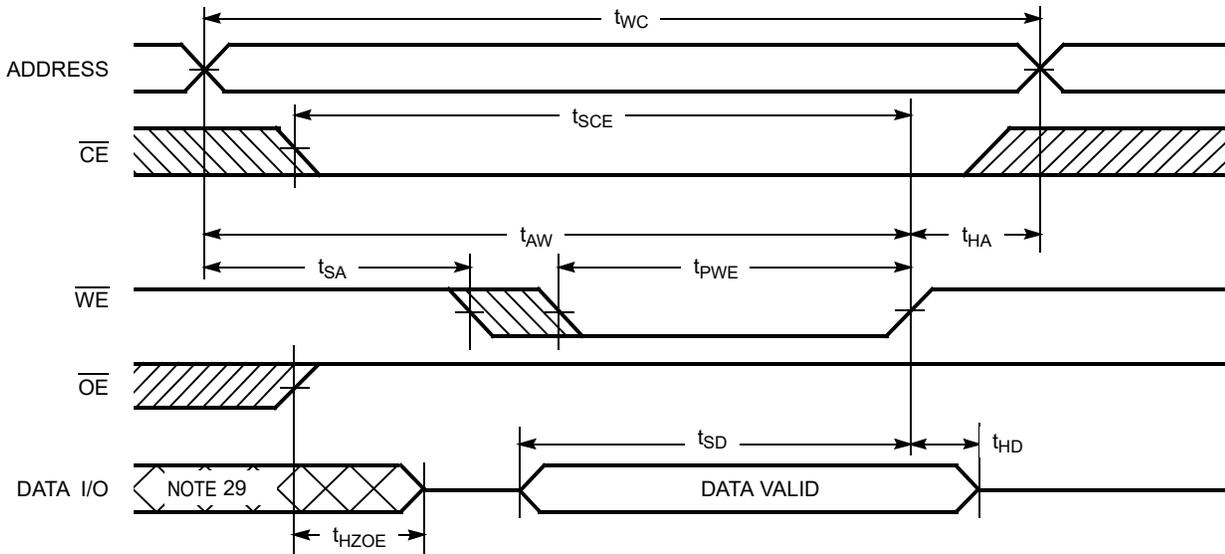
Figure 9. Write Cycle No. 2 ( $\overline{CE}_1$  or  $\overline{CE}_2$  Controlled) [25, 26, 27, 28]
