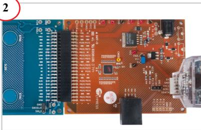
1. Connect the CY3280-SRM board to the CY3280-20x34 UCC board's P2 connector.
